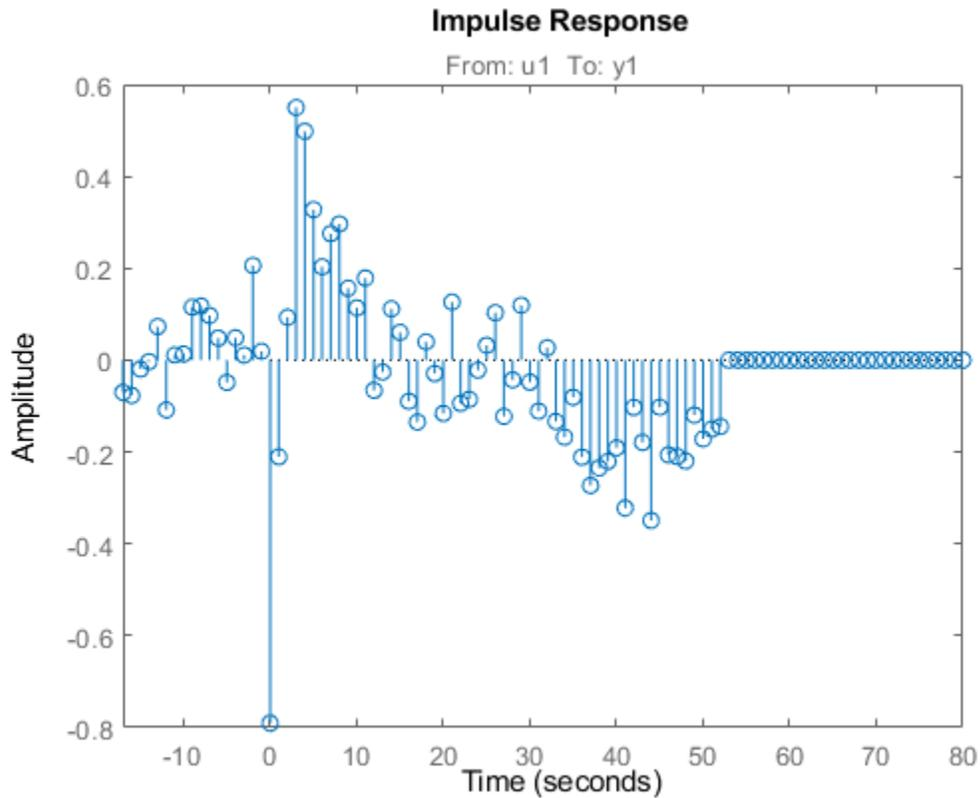
View the zero-response region at one standard deviation by right-clicking on the plot and selecting **Characteristics > Confidence Region**. Alternatively, you can use the `showConfidence` command.
