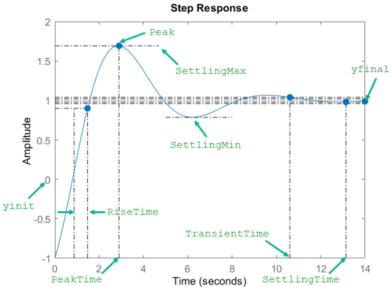
`S = stepinfo(sys)` computes the step-response characteristics for a dynamic system model `sys`. This syntax uses  $y_{init} = 0$  and  $y_{final} =$  steady-state value for computing the characteristics that depend on these values.
