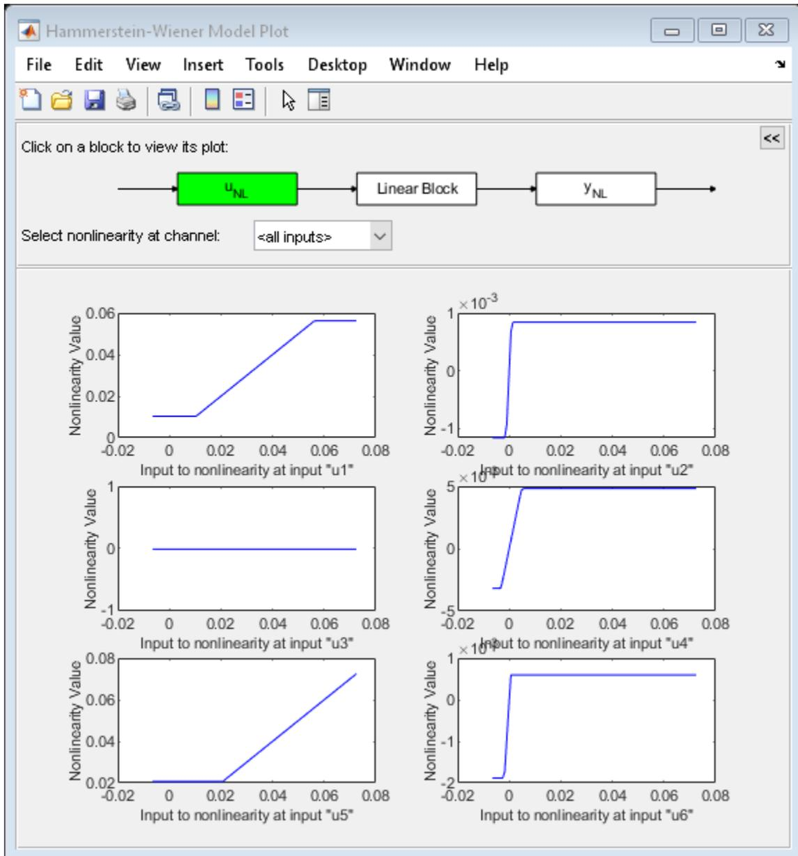
Click on the input and output nonlinearity blocks on the top of the plot to see the nonlinearities.
