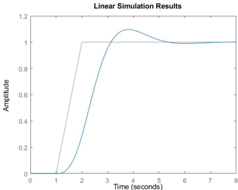
The plot shows the applied input (`u, t`) in gray and the system response in blue.
