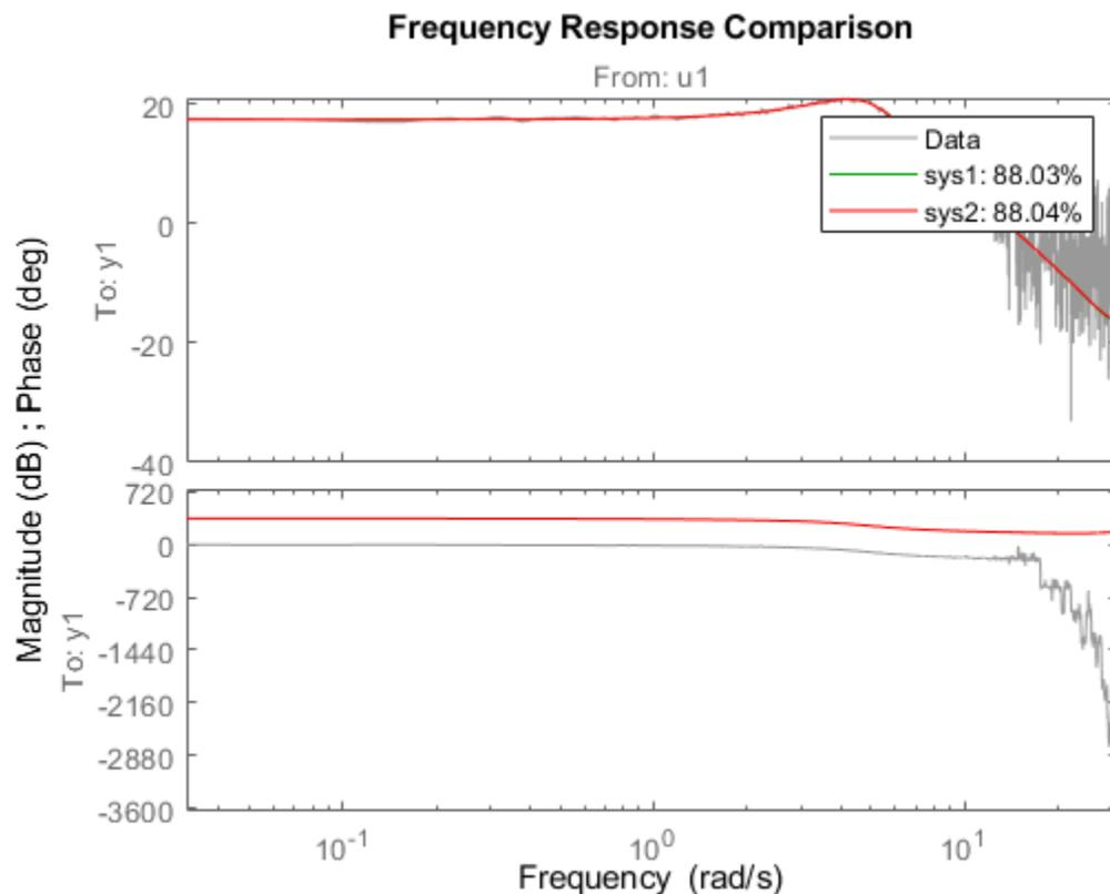
The two models have NRMSE fit values that are nearly equal with respect to the data from which they were calculated.
