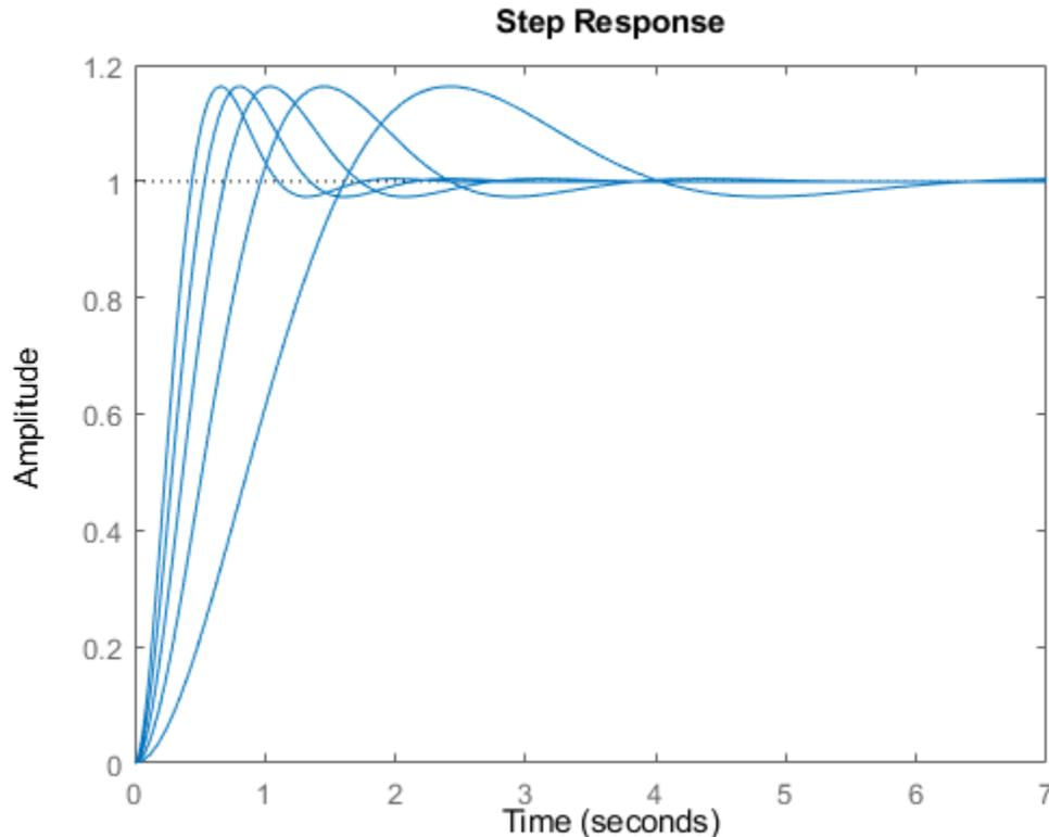
`step` uses the same linestyle for the responses of all entries in the array. One way to distinguish among entries is to use the `SamplingGrid` property of dynamic system models to associate each entry in the array with the corresponding  $w_0$  value.
