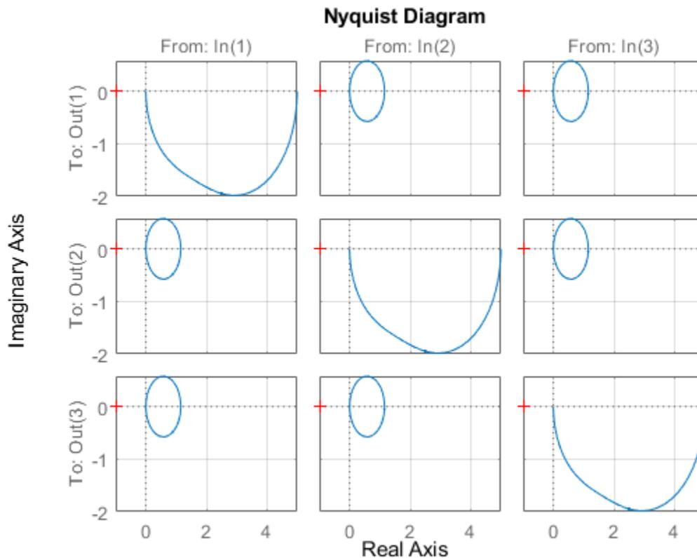
The Nyquist plot automatically updates when you call `setoptions`. For MIMO models, `nyquistplot` produces an array of Nyquist diagrams, each plot displaying the frequency response of one I/O pair.
