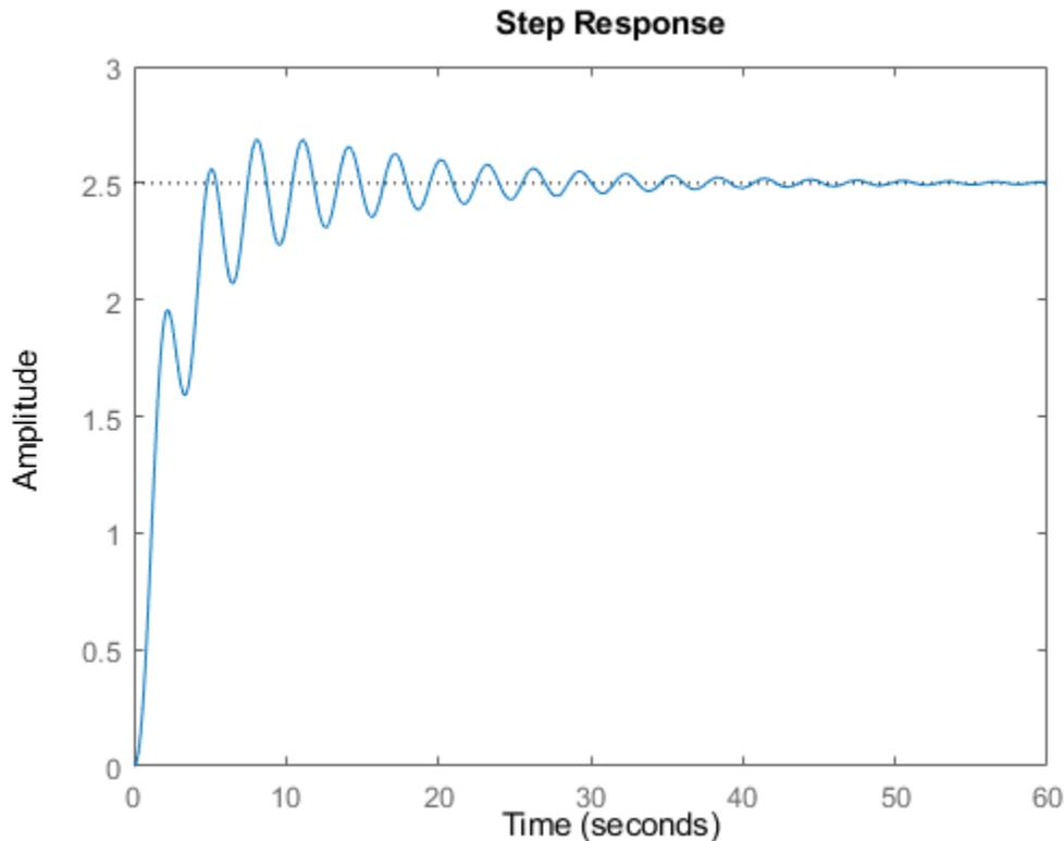
The plot shows that the response rises in a few seconds, and then rings down to a steady-state value of about 2.5. Compute the characteristics of this response using `stepinfo`.
