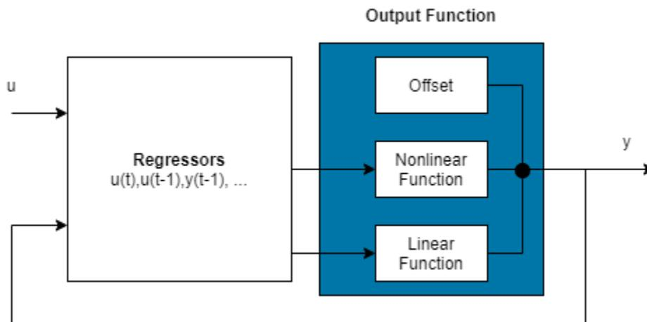
The software computes the nonlinear ARX model output  $y$  in two stages:
