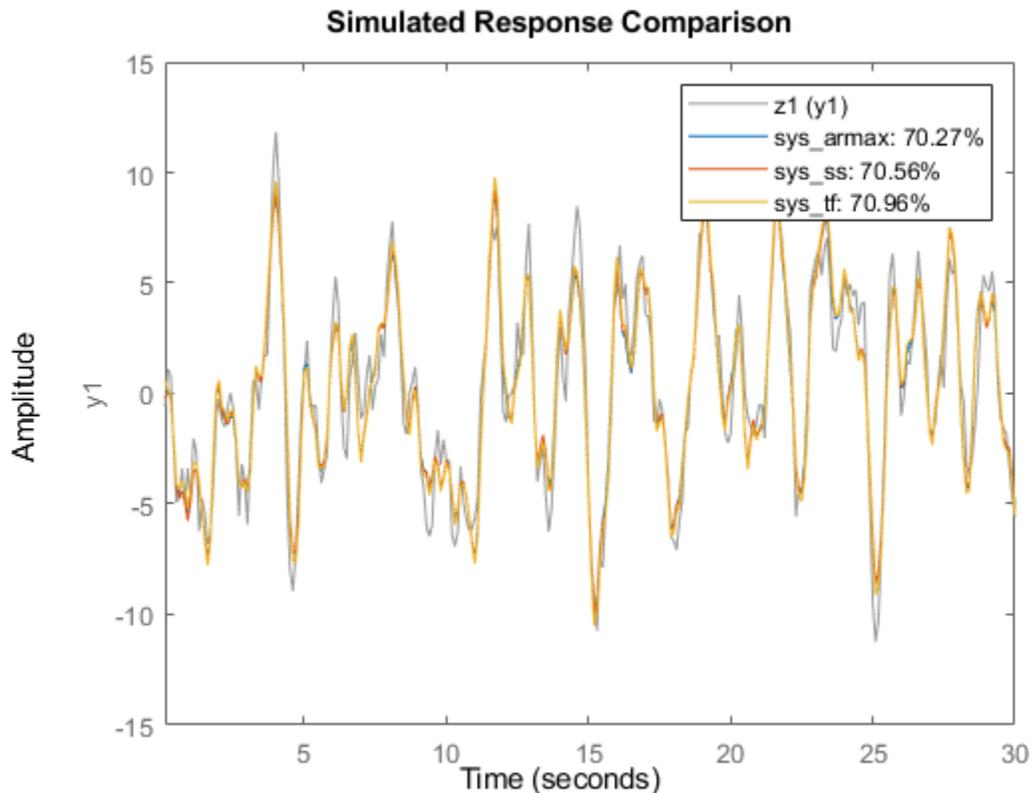
For this set of data, along with the default settings for all the models, the transfer-function form has the best NRMSE fit. However, the fits for all models are within about 1% of each other.
