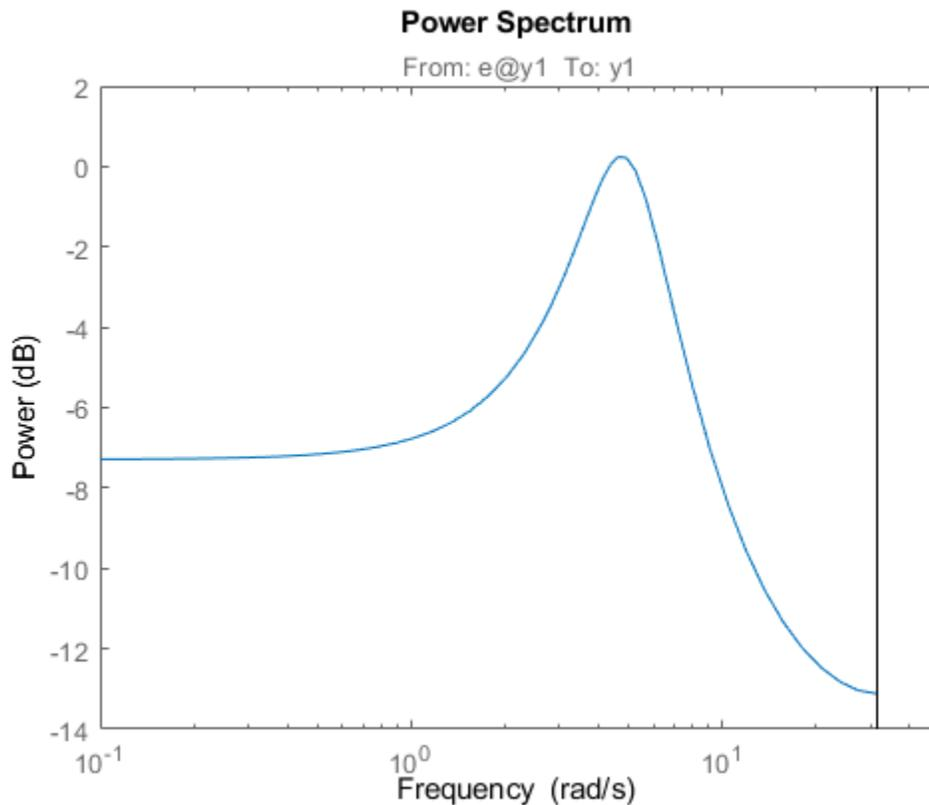
The function plots the spectrum, but limits the frequency range to the Nyquist frequency of approximately 31.4 rad/sec.
