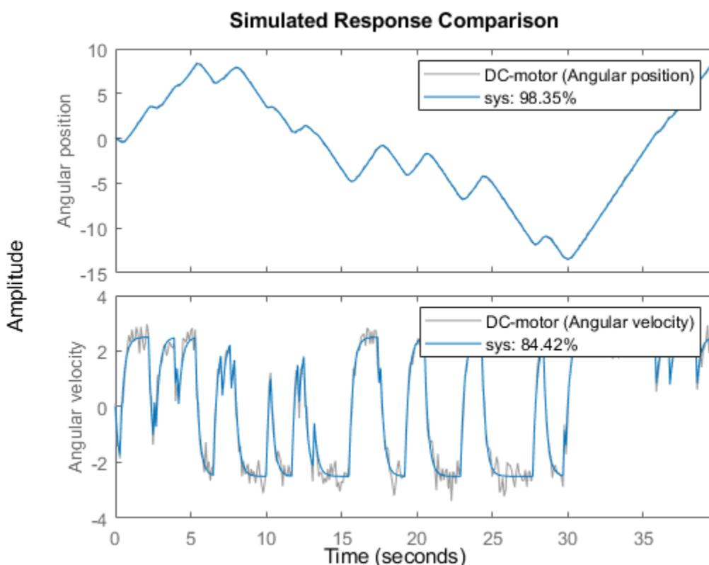
`sys` provides a 98.35% fit for the angular position and an 84.42% fit for the angular velocity.
