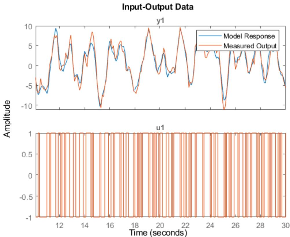
The simulation combines the model response to the input signal with the free response to the initial condition. The measured and simulated outputs now have better agreement at the beginning of the simulation.
