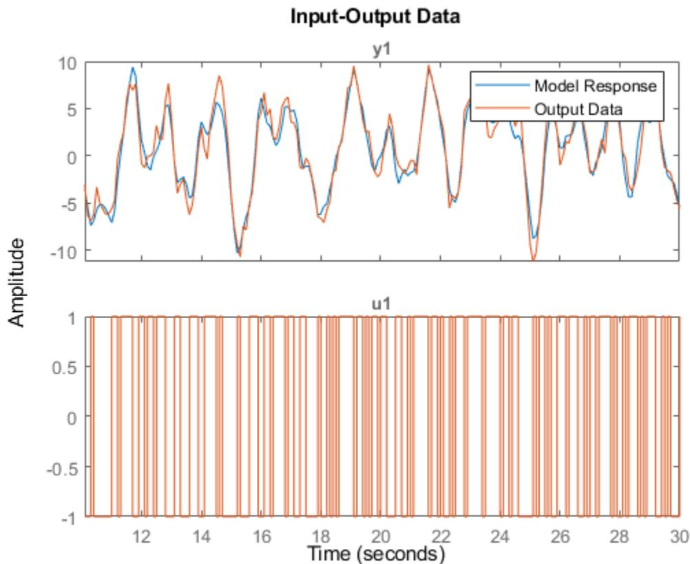
The simulation combines the model response to the input signal with the free response to the initial condition. The measured and simulated outputs now have better agreement at the beginning of the simulation. This initial condition is valid only for the estimation data `z1i`.
