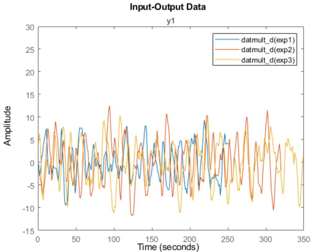
The experimental data are now better aligned, and do not drift significantly away from zero mean.
