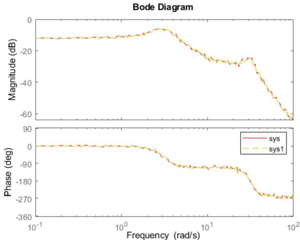
The magnitude and phase of `sys` and `sys1` match because `chgFreqUnit` command changes the units of frequency points in `sys` without modifying system behavior.
