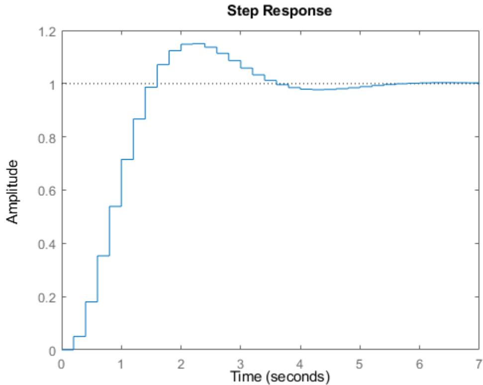
The step response reflects the discretization of the model, showing the response computed every 0.2 seconds.
