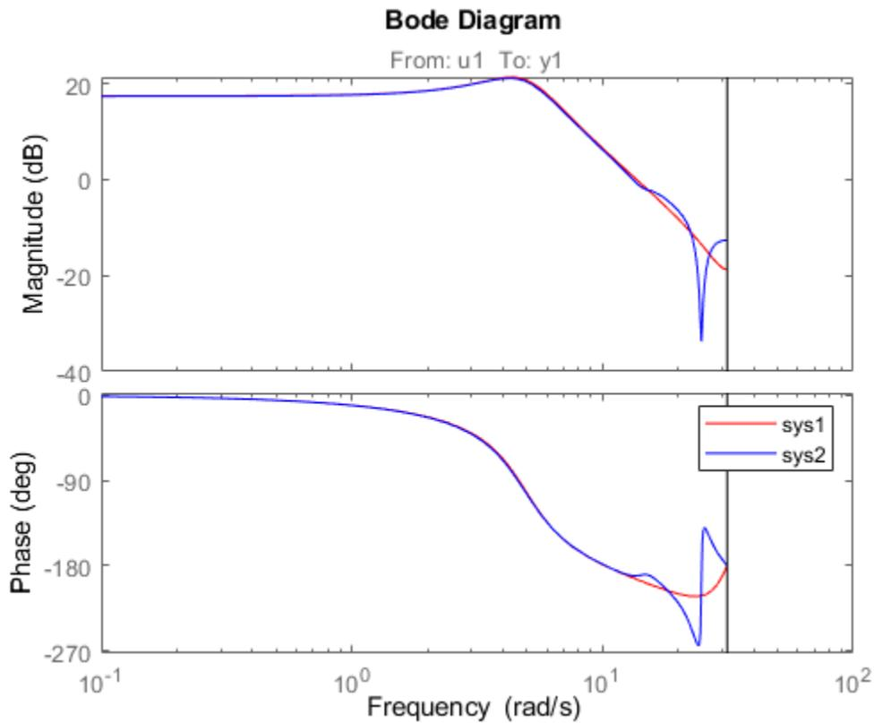
From the plot, observe that both models produce about 70% fit to data. However, `sys2` shows higher uncertainty in its frequency response, especially close to the Nyquist frequency. Now, use `linspace` to create a vector of frequencies and plot the Bode response using the frequency vector `w`.
