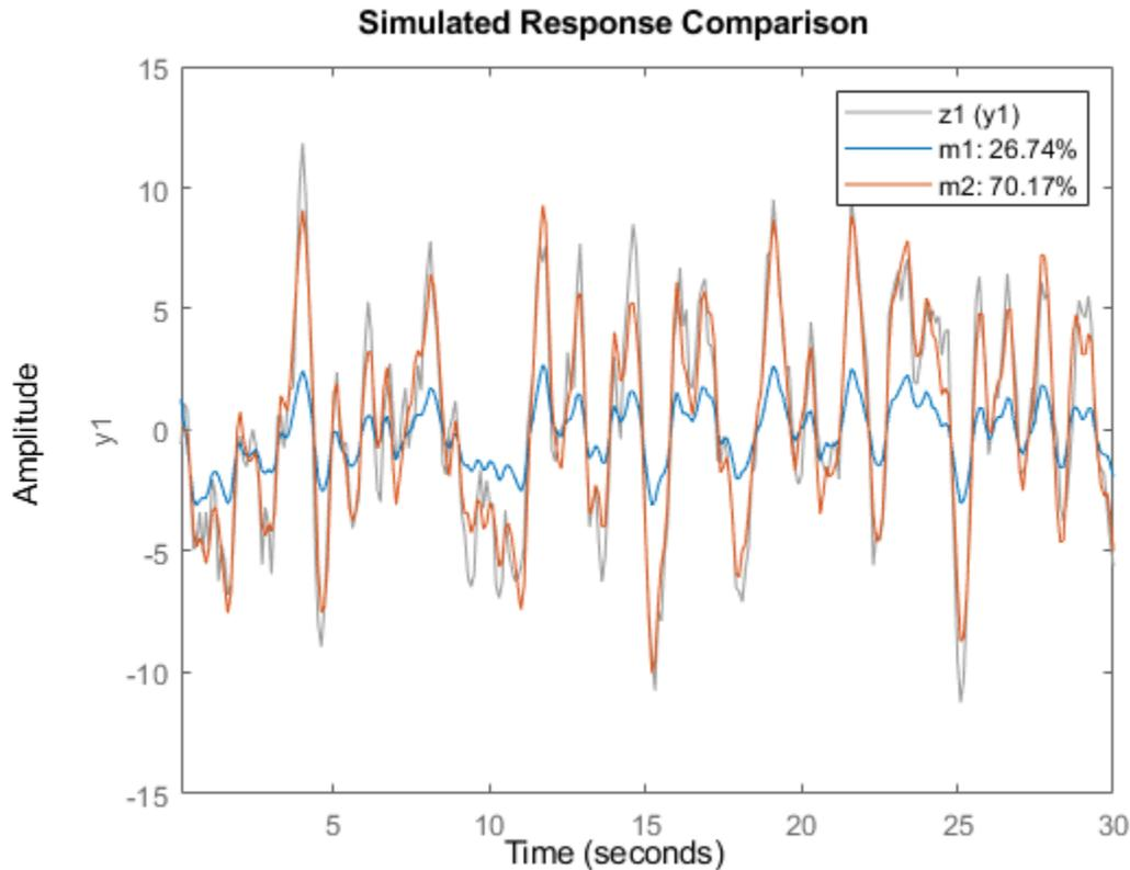
Regularization helps steer the estimation process towards the correct parameter values.
