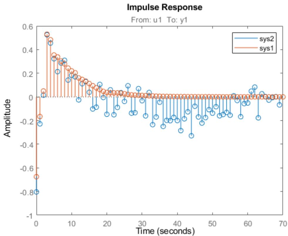
As the plot shows, using regularization makes the response smoother.
