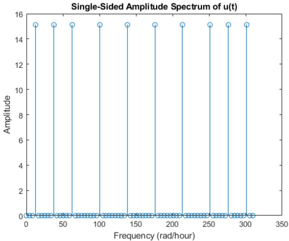
The generated plot shows the frequencies of the 10 sine waves used to generate the signal. For example, the plot shows that the first sine wave has a frequency of 12.57 rad/hour, the same as `freq(1)`.
