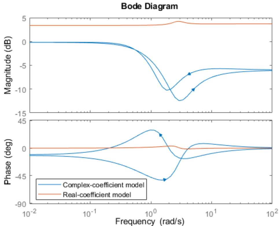
In log frequency scale, the plot shows two branches for complex-coefficient models, one for positive frequencies, with a right-pointing arrow, and one for negative frequencies, with a left-pointing arrow. In both branches, the arrows indicate the direction of increasing frequencies. The plots for real-coefficient models always contain a single branch with no arrows.
