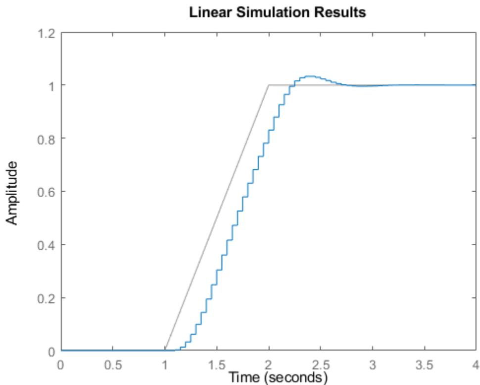
To simulate the response of a discrete-time system to a periodic input signal, use the same sample time with `gensig` to generate the input. For instance, simulate the system response to a sine wave with period of 1 s and a duration of 4 s.
