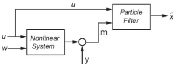
The algorithm computes the state estimates  $\hat{x}$  of the nonlinear system using the state transition and measurement likelihood functions you specify.
