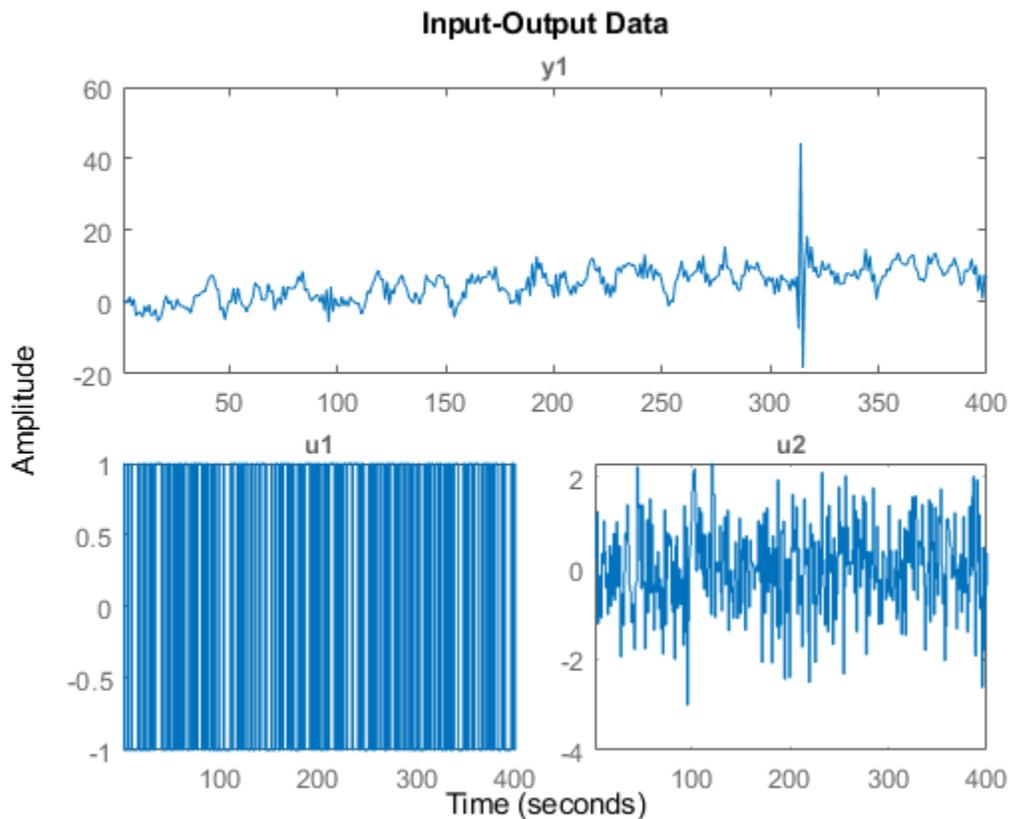
The output channel of z7L contains a linear trend that is not present in the input channels. Compute the trend information.
