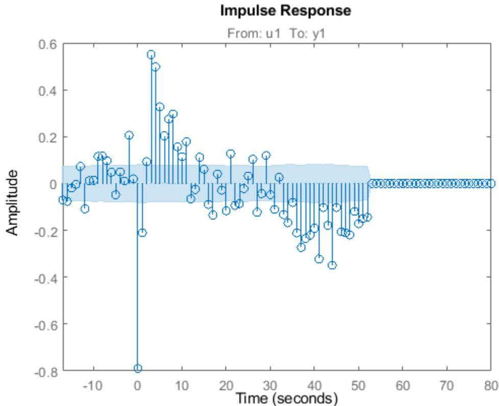
The large response value at  $t=0$  (zero lag) suggests that the data comes from a process containing feedthrough. That is, the input affects the output instantaneously. The large response value can also indicate direct feedback, such as proportional control without some delay so that  $y(t)$  partly determines  $u(t)$ .
