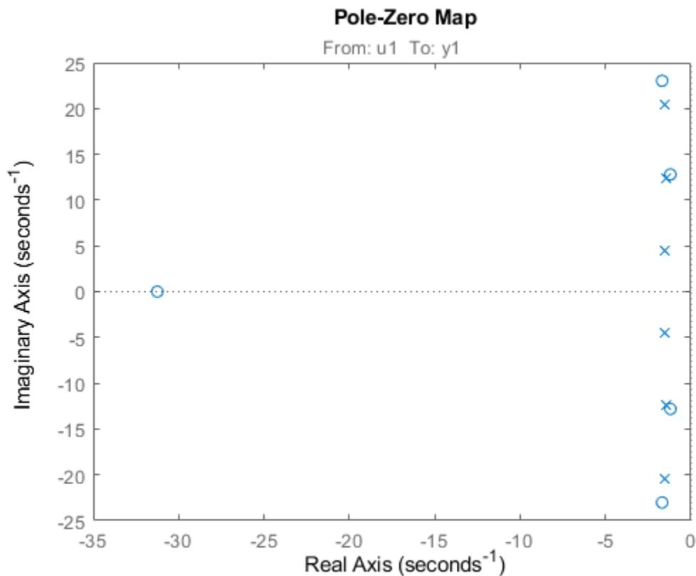
The plot shows that there are two pole-zero pairs that almost overlap, which hints are their potential redundancy.
