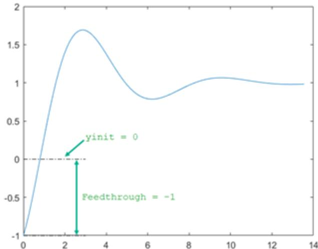
Here,  $y_{init}$  is zero and the feedthrough value is -1.
