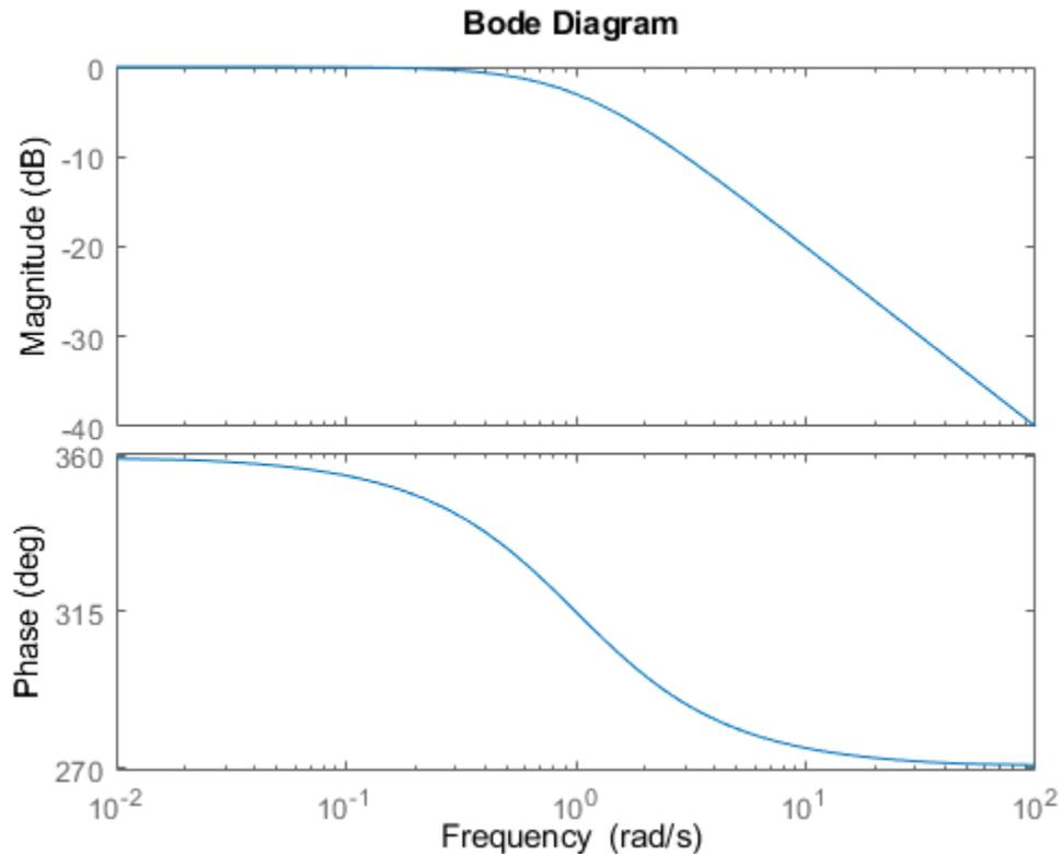
The first bode plot has a phase of -45 degrees at a frequency of 1 rad/s. Setting the phase matching options so that at 1 rad/s the phase is near 150 degrees yields the second Bode plot. Note that, however, the phase can only be  $-45 + N \cdot 360$ , where  $N$  is an integer. So the plot is set to the nearest allowable phase, namely 315 degrees (or  $1 \cdot 360 - 45 = 315^\circ$ ).
