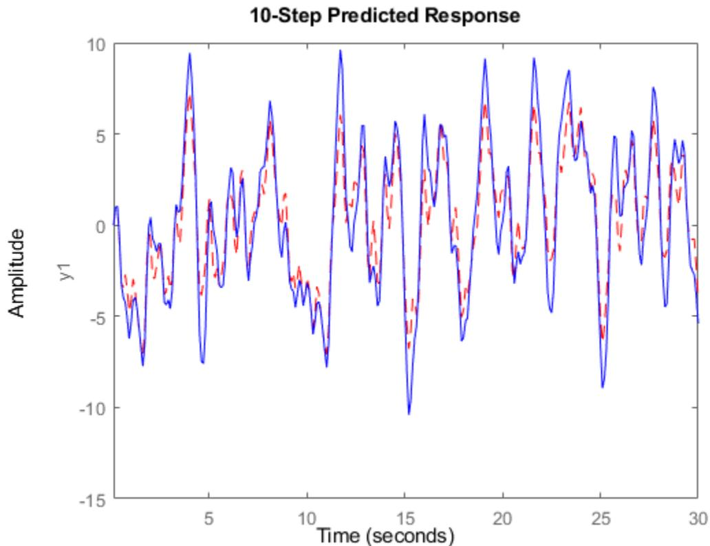
To change the display options, right-click the plot to access the context menu. For example, to view the estimation data, select **Show Validation Data** from the context menu. To view the prediction error, select **Prediction Error Plot**.
