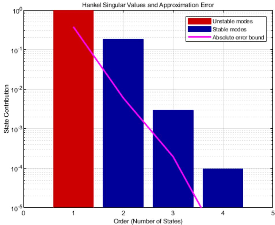
Observe that the first HSV is red which indicates that it is associated with an unstable mode.
