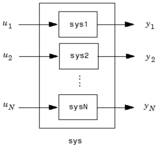
For systems with transfer functions  $H_1(s), \dots, H_N(s)$ , the resulting system `sys` has the block-diagonal transfer function
