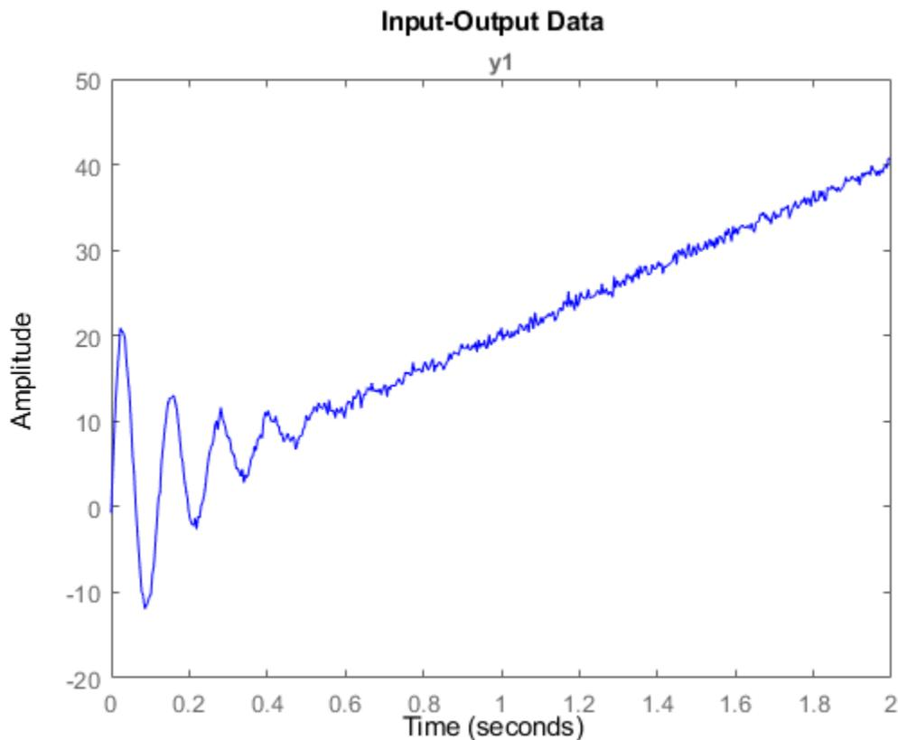
The plot shows a clear linear trend in the data. Use `detrend` linear option (`Type = 1`) to subtract the trend from the data. `detrend` fits the data and determines the linear trend to subtract. Include the `TrendInfo` object `Tr` as an output argument so you can see what `detrend` subtracts.
