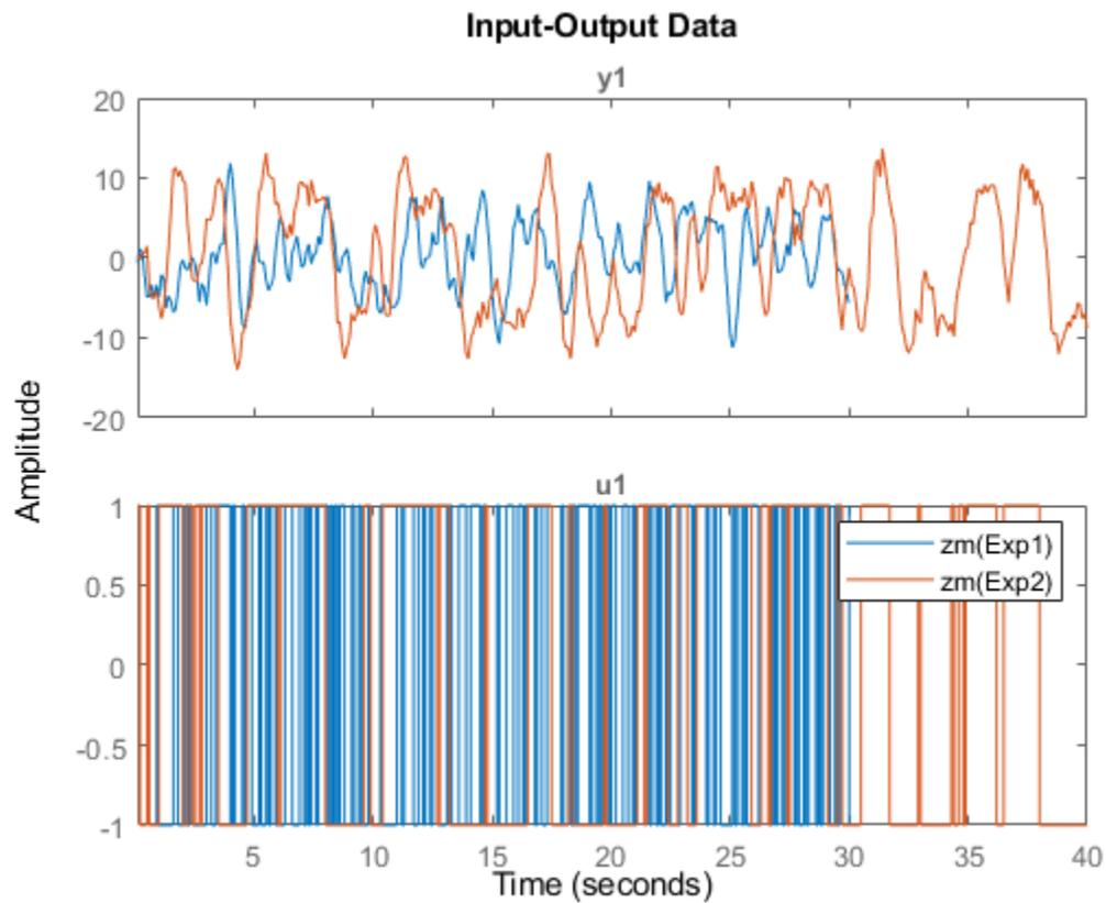
For multiexperiment data, each experiment is treated as a separate data set. You can right-click the plots to view their characteristics.
