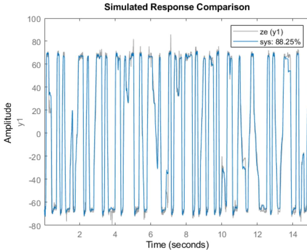
Compare the model simulated output to the validation data output.
