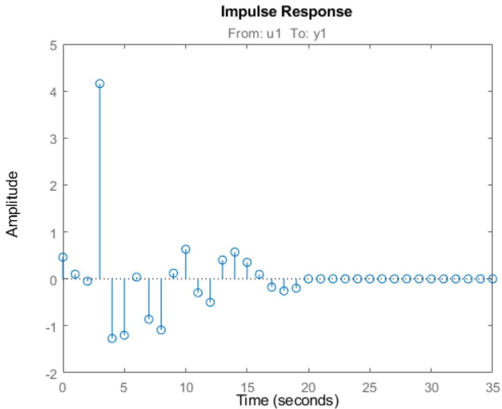
The plot shows that the impulse response includes nonzero samples during the 3-second delay period.
