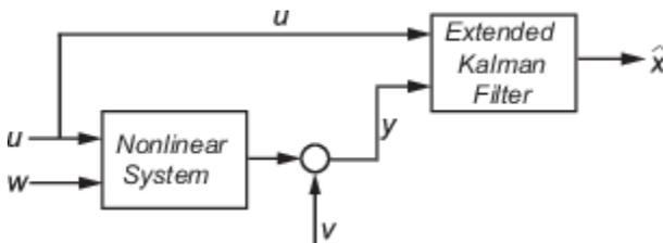
Using the state transition and measurement functions of the system and the extended Kalman filter algorithm, the block produces state estimates  $\hat{x}$  for the current time step. For information about the algorithm, see “Extended and Unscented Kalman Filter Algorithms for Online State Estimation”.
