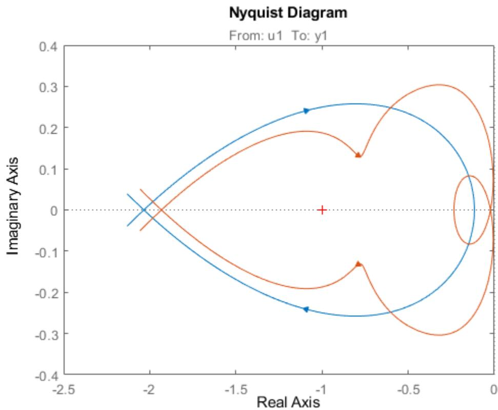
Both models produce about 76% fit to data. However, `sys2` shows higher uncertainty in its frequency response, especially close to Nyquist frequency as shown by the plot. To see this, show the confidence region at a subset of the points at which the Nyquist response is displayed.
