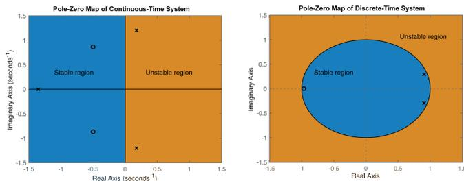
From the figure above, an open-loop linear time-invariant system is stable if:
