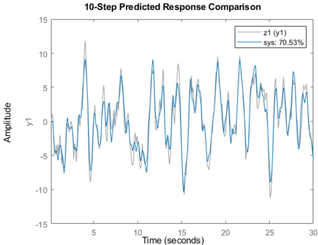
In this plot, each `sys` data point represents the predicted output associated with output measurement data that was taken at least 10 steps earlier. For instance, the point at  $t = 15$  s is based on output measurements taken at or prior to  $t = 5$  s. The calculation of this  $t = 15$  s `sys` data point also uses input measurements up to  $t = 15$  s, just as a simulation would.
