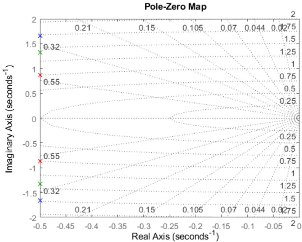
sgrid plots lines of constant damping ratio and natural frequency in the s-plane of the pole-zero plot.
