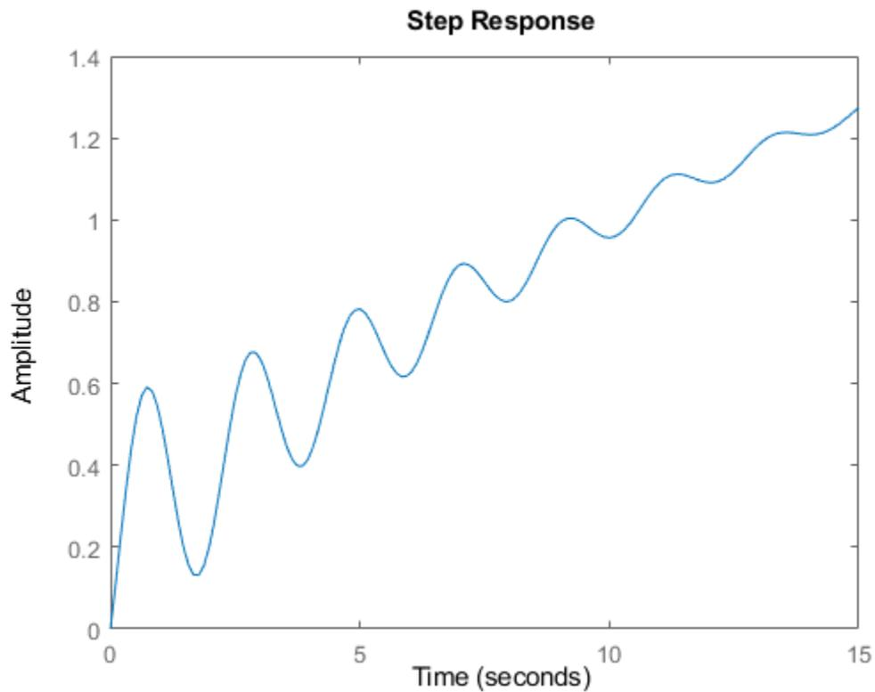
Alternatively, you can specify the exact times at which you want to examine the step response, provided they are separated by a constant interval. For instance, examine the response from the end of the transient until the system reaches steady state.
