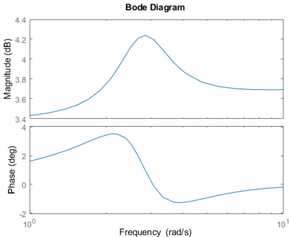
Change the units to Hz and suppress the phase plot. To do so, edit properties of the plot handle, `h` using `setoptions`.
