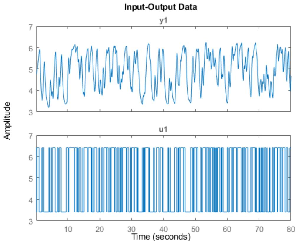
The known offset of 4 (from operating point 1) is visible in the plots. You can construct a `TrendInfo` object to capture this offset, using the function `getTrend`.
