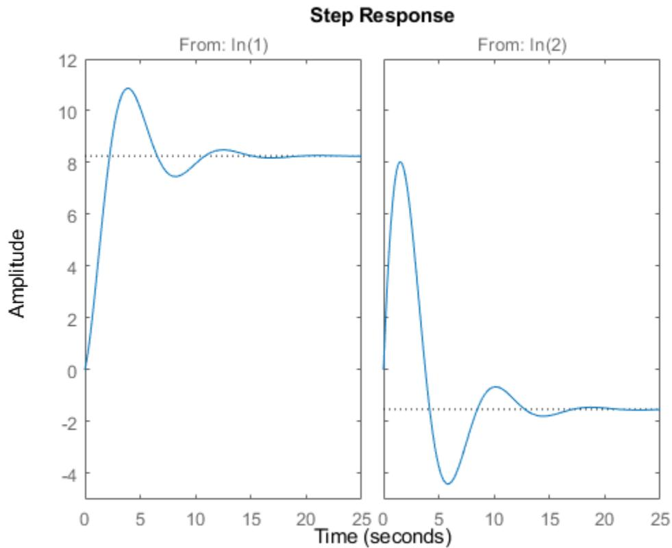
The left plot shows the step response of the first input channel, and the right plot shows the step response of the second input channel. Whenever you use `step` to plot the responses of a MIMO model, it generates an array of plots representing all the I/O channels of the model. For instance, create a random state-space model with five states, three inputs, and two outputs, and plot its step response.
