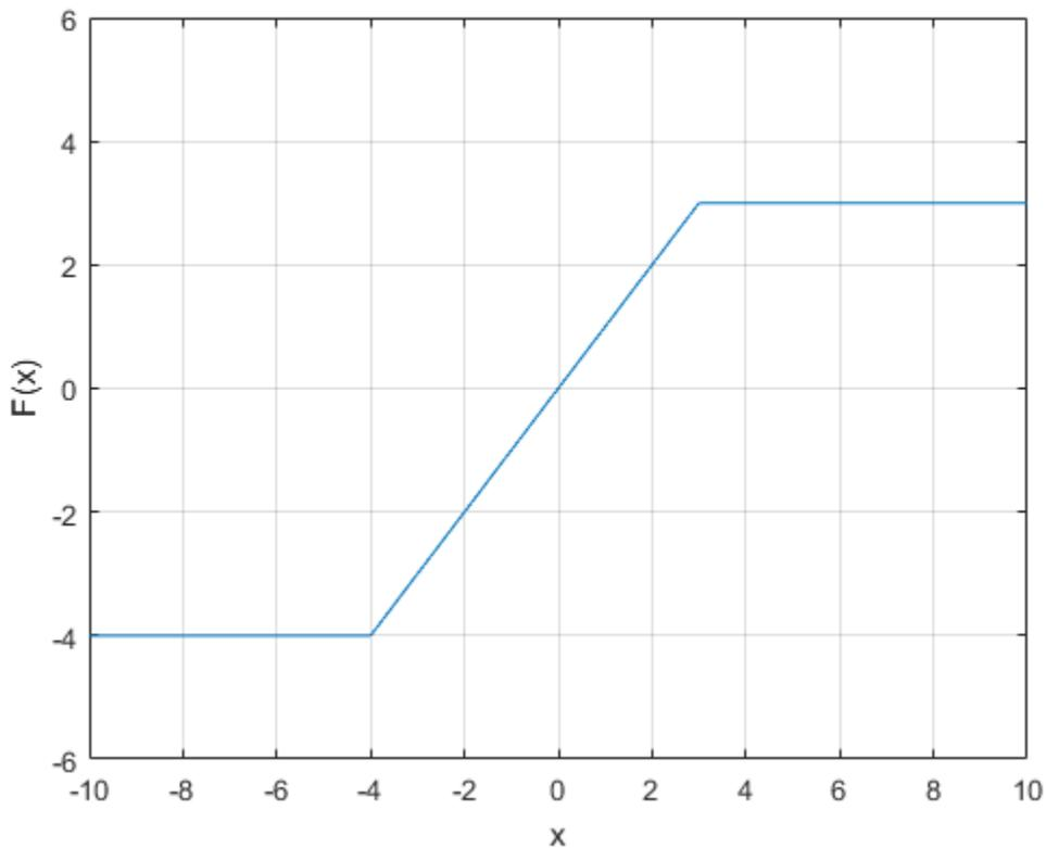
The value  $F(x)$  is computed by `evaluate(NL,x)`, where `NL` is the `idSaturation` object. For `idSaturation` object properties, see “Properties” on page 1-705.
