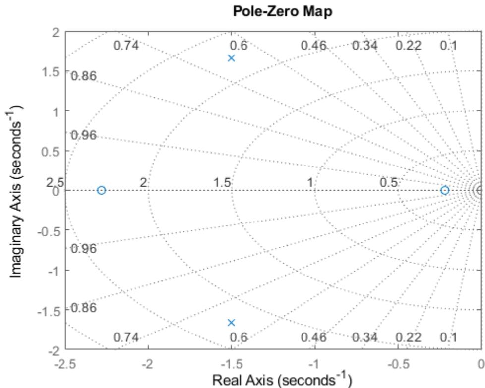
Turning on the grid displays lines of constant damping ratio ( $\zeta$ ) and lines of constant natural frequency ( $\omega_n$ ). This system has two real zeros, marked by o on the plot. The system also has a pair of complex poles, marked by x.
