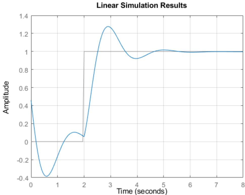
The first half of the plot shows the free evolution of the system from the initial state values  $[-0.2 \ 0.3]$ . At  $t = 2$  there is a step change to the input, and the plot shows the system response to this new signal beginning from the state values at that time.
