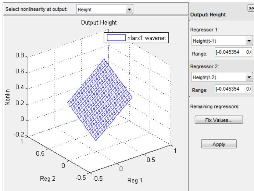
To understand what is plotted, suppose that  $\{r_1, r_2, \dots, r_N\}$  are the *N* regressors used by a nonlinear ARX model *M* with nonlinearity *nl* corresponding to a model output. You can use `getreg(M)` to view these regressors. The expression `Nonlin = evaluate(nl, [v1, v2, ..., vN])` returns the model
