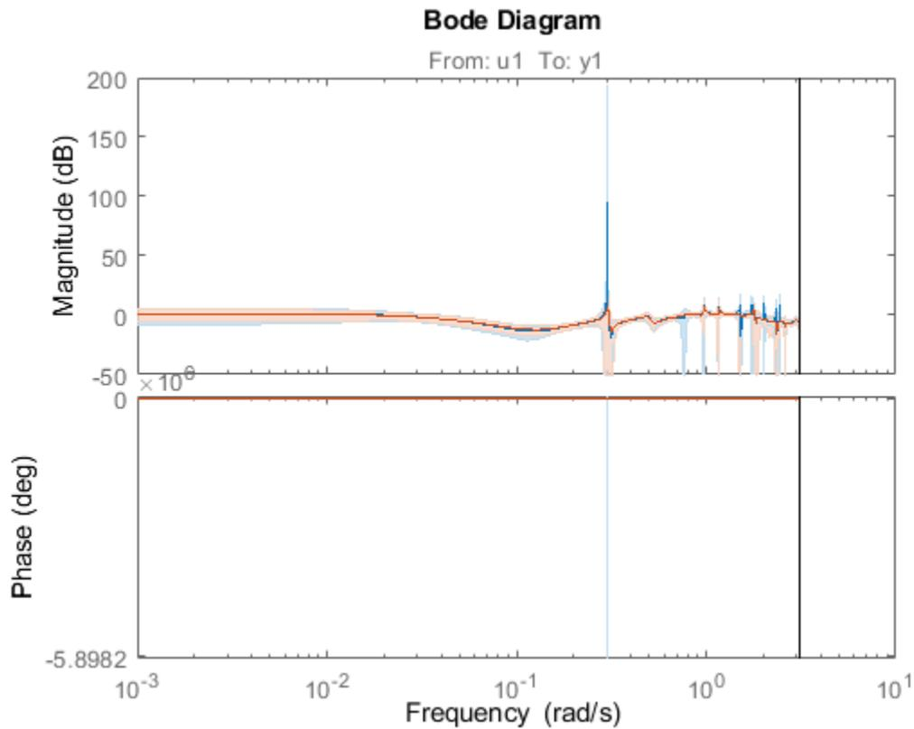
The regularized model `m2` has a reduced variance compared to the unregularized model `m1`.
