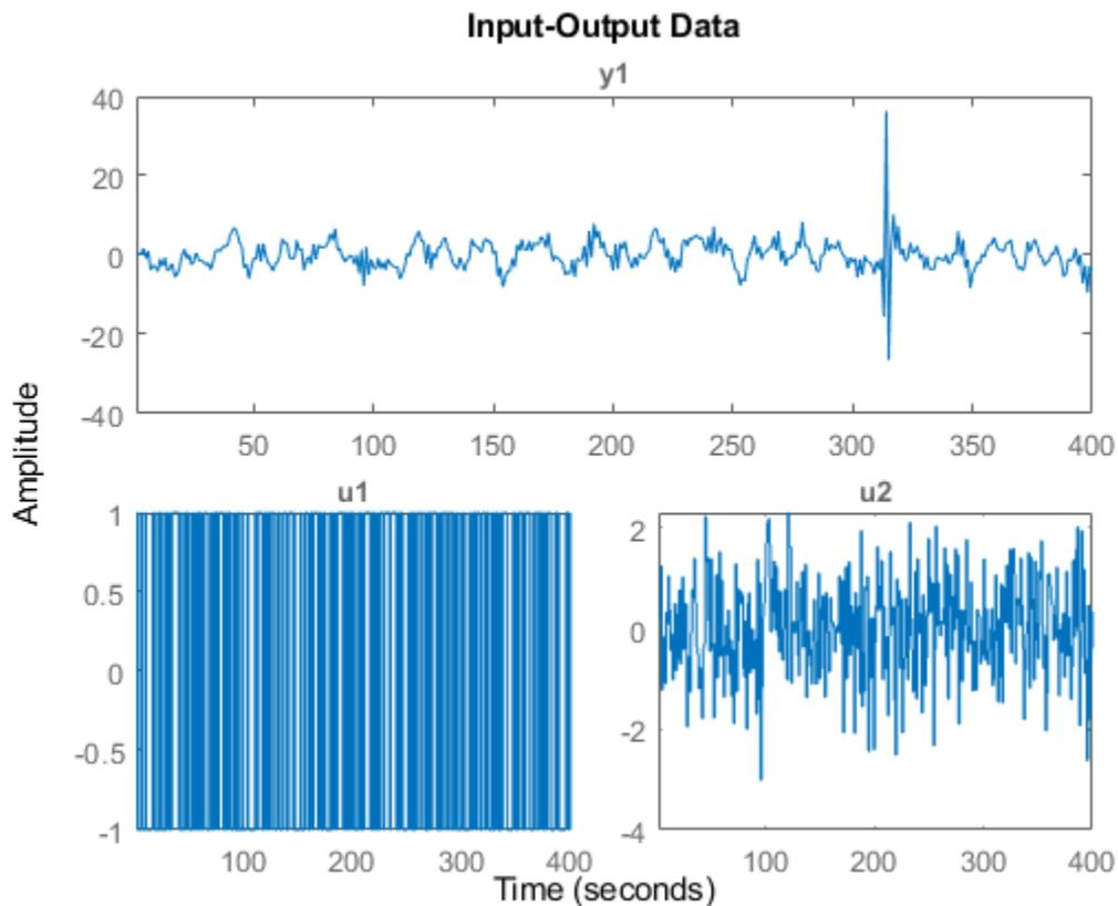
The trend is no longer in the output data and the input data is unchanged.
