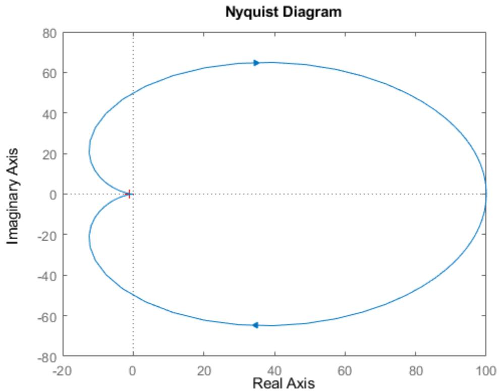
Zoom in on the critical point,  $(-1,0)$ . You can do so interactively by right-clicking on the plot and selecting **Zoom on  $(-1,0)$** . Alternatively, use the `zoomcp` command on the plot handle `h`.
