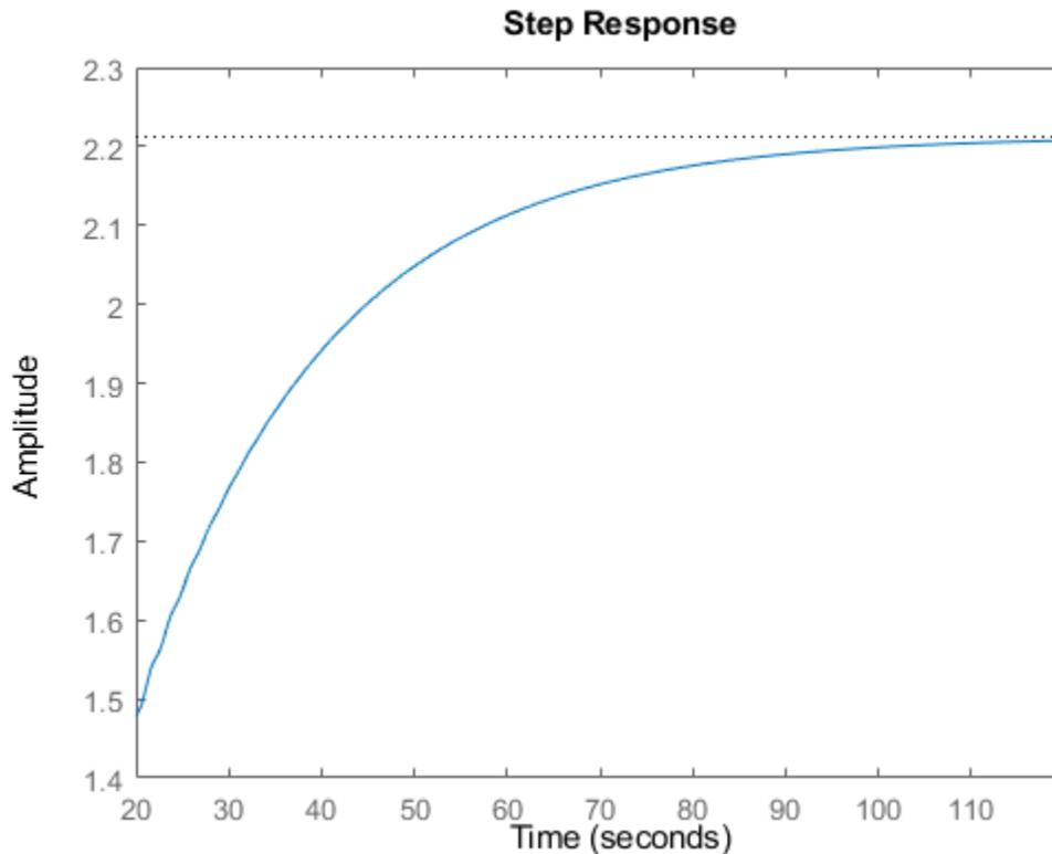
Even though this plot begins at  $t = 20$ , `step` always applies the step input at  $t = 0$ .
