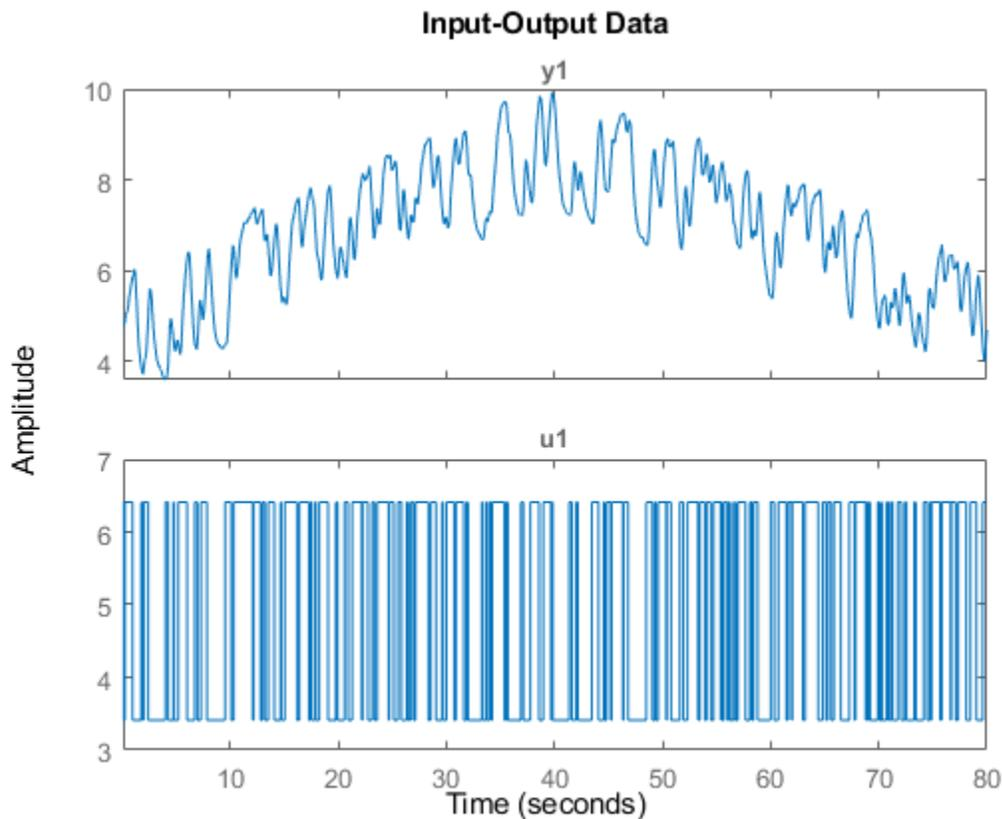
Both input and output plots show a bias. However, the output plot also shows an inverted V-shape trend that is not present in the input data.
