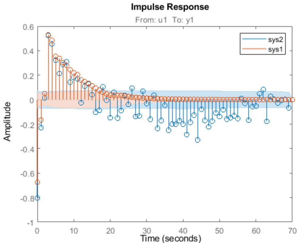
The uncertainty in the computed response is reduced at larger lags for the model using regularization. Regularization decreases variance at the price of some bias. The tuning of the 'TC' regularization is such that the variance error dominates the overall error.
