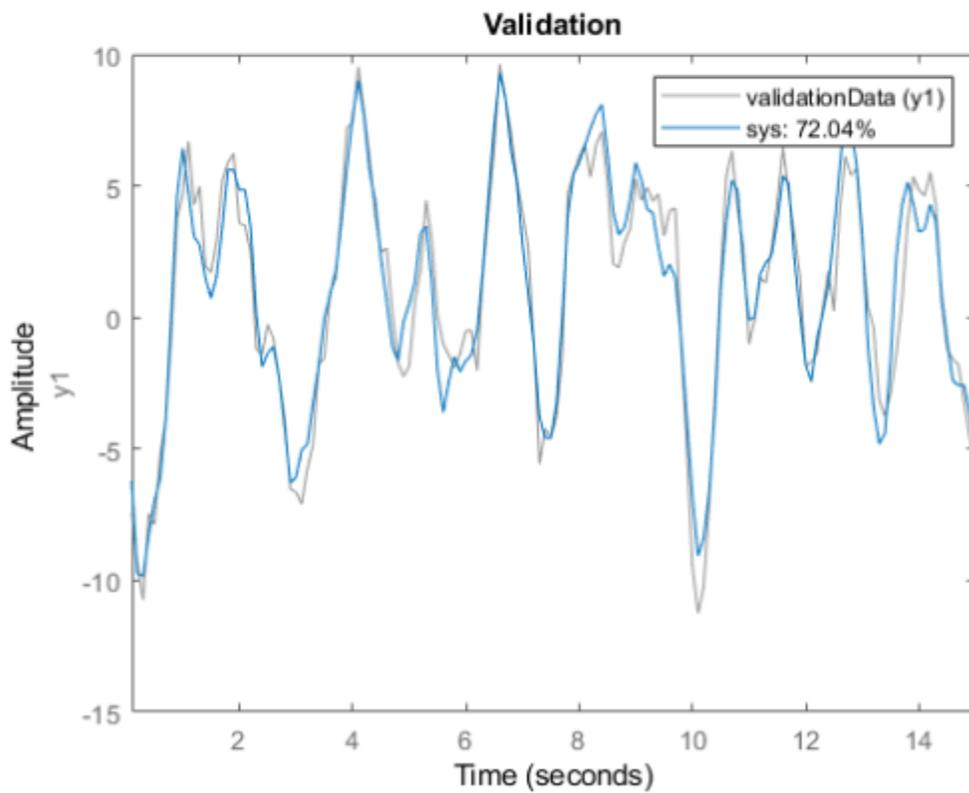
The fit to the estimation data is somewhat worse than in “Estimate State-Space Model with Live Editor Task” on page 1-302. Estimation in the current example has only half the data with which to estimate the model. The fit to the validation data, which represents the goodness of the model more generally, is better than the fit to the estimation data.
