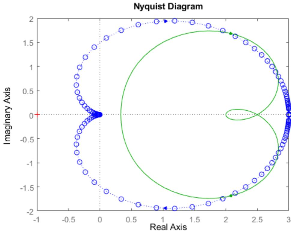
The first LineSpec, 'o:', specifies a dotted line with circle markers for the response of sys1. The second LineSpec, 'g', specifies a solid green line for the response of sys2.
