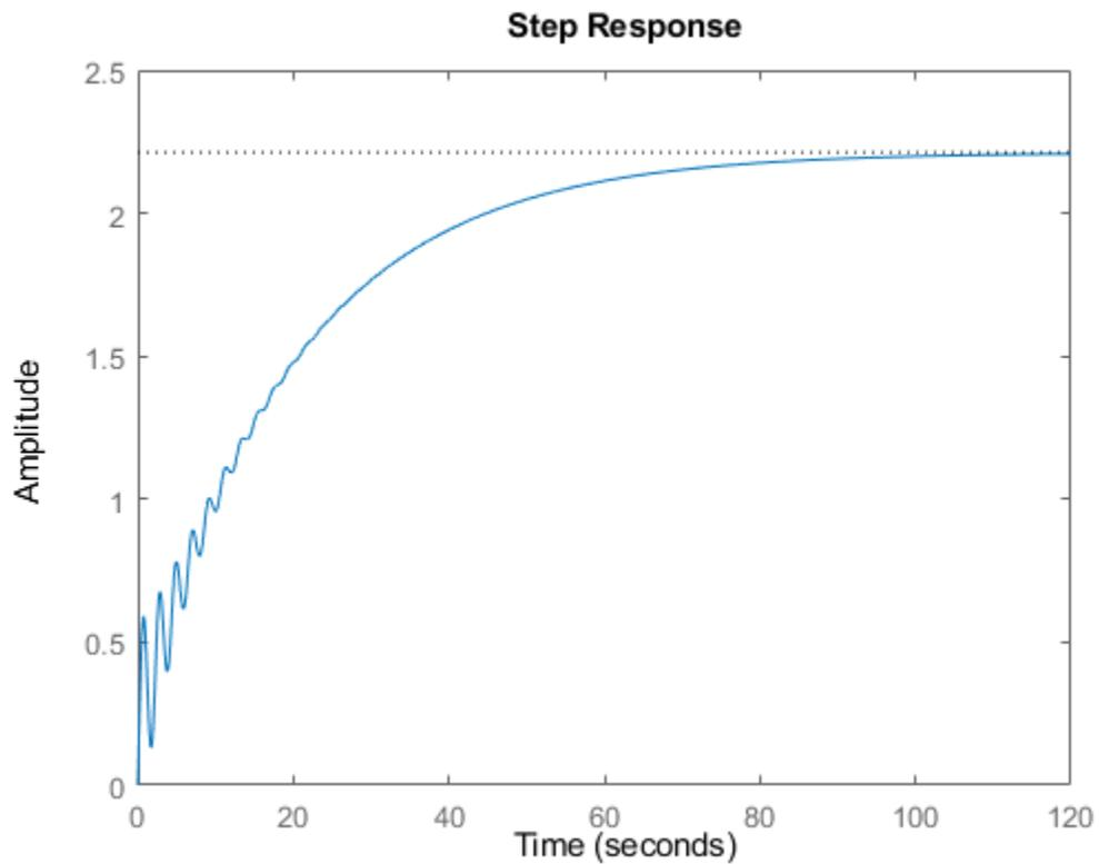
By default, `step` chooses an end time that shows the steady state that the response is trending toward. This system has fast transients, however, which are obscured on this time scale. To get a closer look at the transient response, limit the step plot to  $t = 15$  s.
