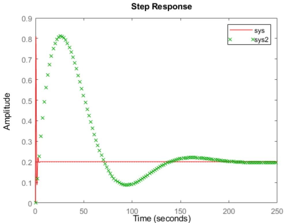
The step responses of `sys` and `sys2` do not match. For example, the original rise time of 0.04 seconds changes to 0.04 minutes.
