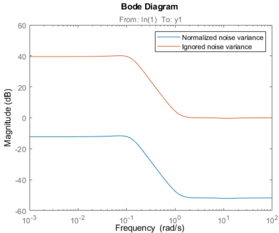
The difference between the bode magnitudes of the `noise_model_innovation` and `noise_model_normalize` is approximately 51 dB. As expected, the magnitude difference is approximately equal to  $20 \cdot \log_{10}(L)$ .
