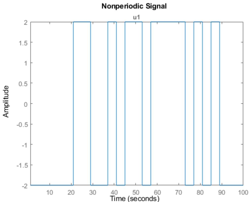
The generated signal is a nonperiodic PRBS of length 100. The signal remains constant for at least 4 samples before each change in value. Thus, the signal satisfies the clock period specified in Band.
