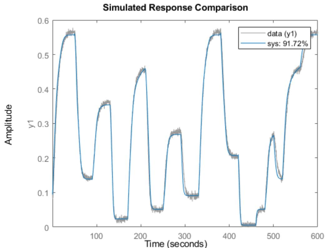
The plot shows good agreement between the measured signal and the simulated model output signal.
