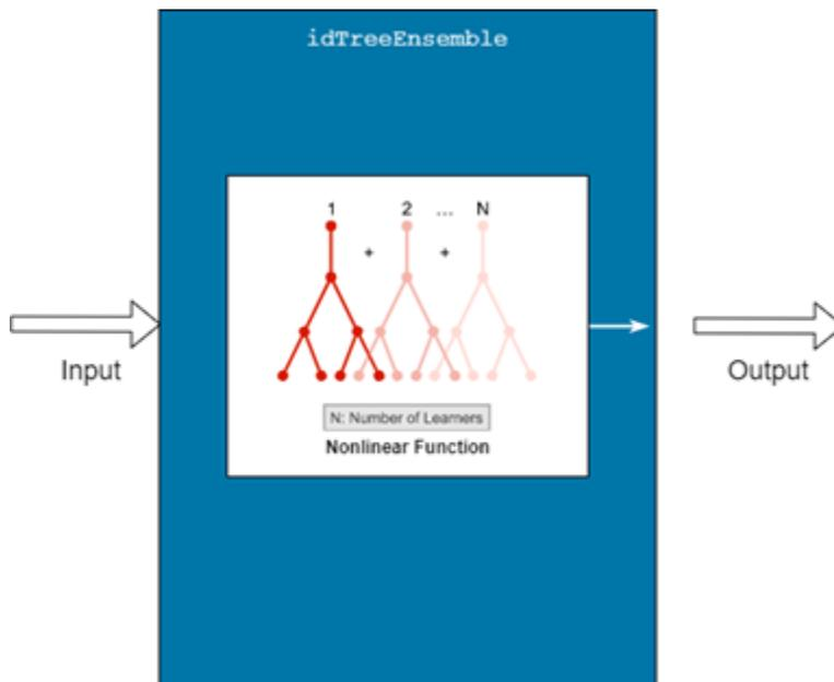
Mathematically, the `idTreeEnsemble` object maps  $m$  inputs  $x(t) = [x_1(t), x_2(t), \dots, x_m(t)]^T$  to a scalar output  $y(t)$  using a decision tree regression ensemble model.
