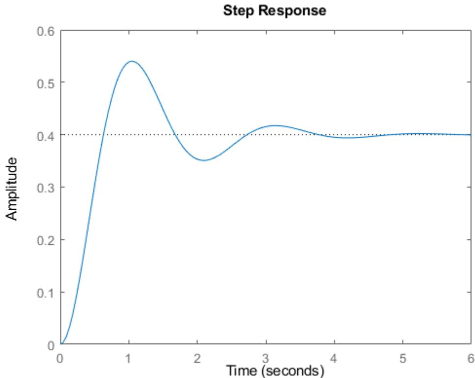
The step plot automatically includes a dotted horizontal line indicating the steady-state response. In a MATLAB® figure window, you can right-click on the plot to view other step-response characteristics such as peak response and settling time. For more information about these characteristics, see `stepinfo` (Control System Toolbox).
