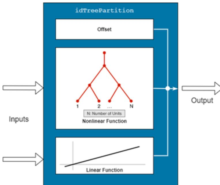
Mathematically, `idTreePartition` is a nonlinear function  $y = F(x)$  that maps  $m$  inputs  $X(t) = [x(t_1), x_2(t), \dots, x_m(t)]^T$  to a scalar output  $y(t)$ .  $F$  is a piecewise-linear (affine) function of  $x$ :
