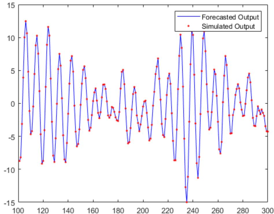
Simulation of forecasting model, `sysf`, with inputs, `future_inputs`, and initial conditions, `x0`, yields the forecasted output, `yf`.
