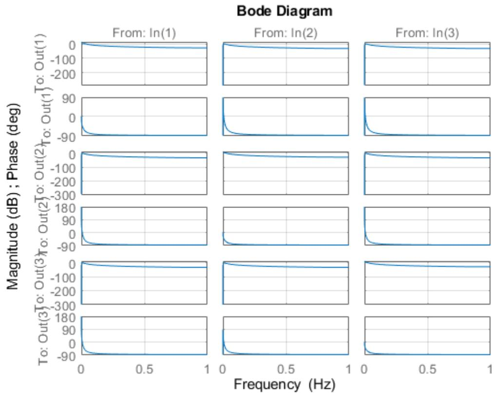
The Bode plot automatically updates when you call `setoptions`. For MIMO models, `bodeplot` produces an array of Bode plots, each plot displaying the frequency response of one I/O pair.
