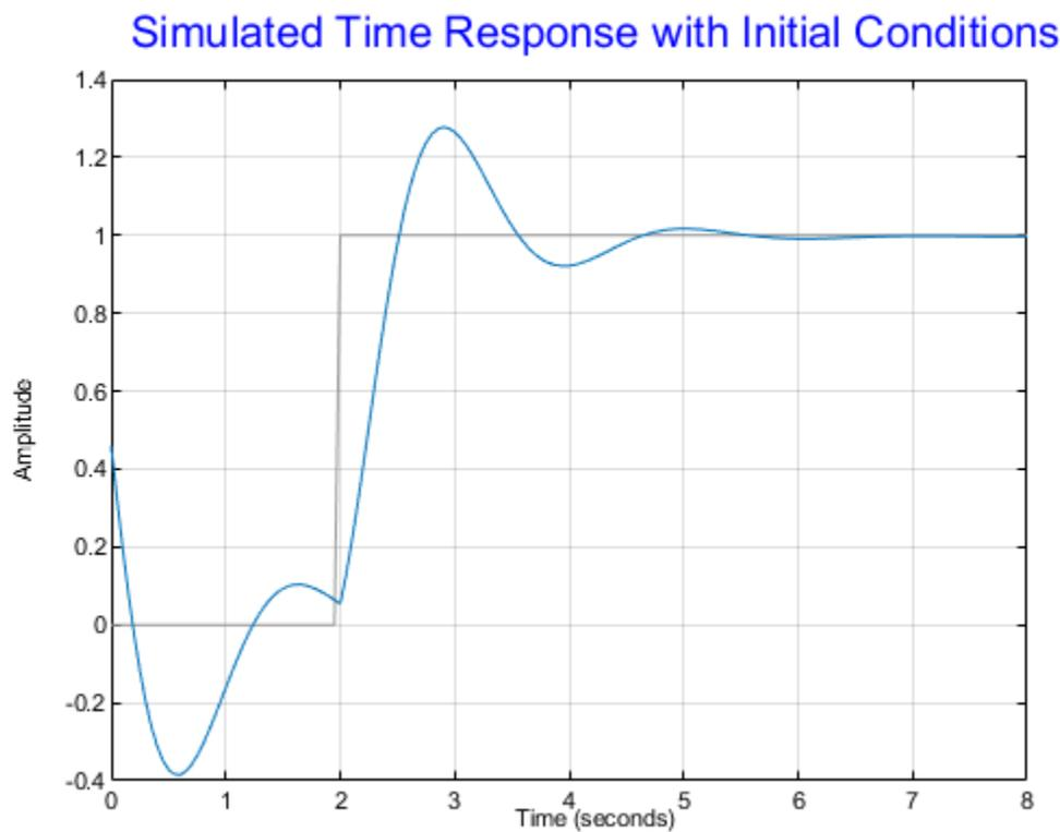
The first half of the plot shows the free evolution of the system from the initial state values  $[-0.2 \ 0.3]$ . At  $t = 2$  there is a step change to the input, and the plot shows the system response to this new signal beginning from the state values at that time. Because `plotoptions` begins with a fixed set of options, the plot result is independent of the toolbox preferences of the MATLAB session.
