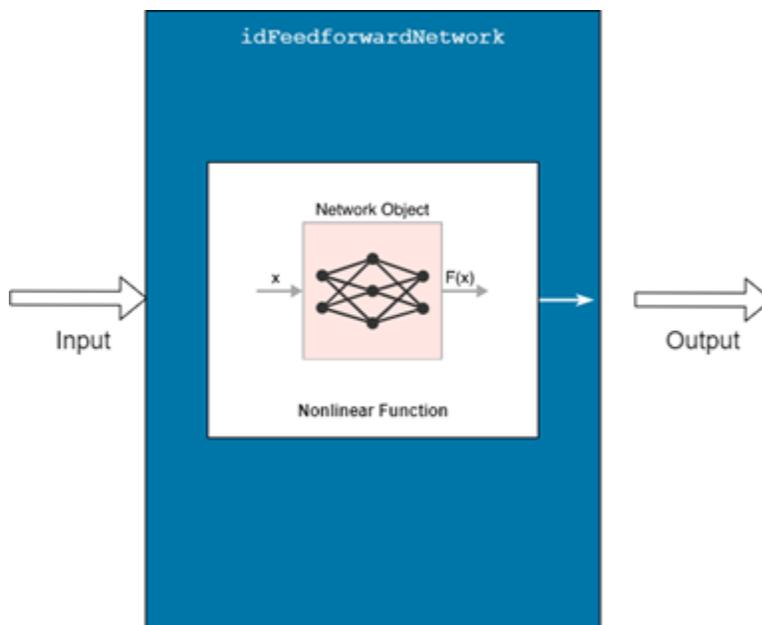
Mathematically, `idFeedforwardNetwork` is a function that maps  $m$  inputs  $X(t) = [x_1(t), x_2(t), \dots, x_m(t)]^T$  to a scalar output  $y(t)$ , using a multilayer feedforward (static) neural network, as defined in Deep Learning Toolbox.
