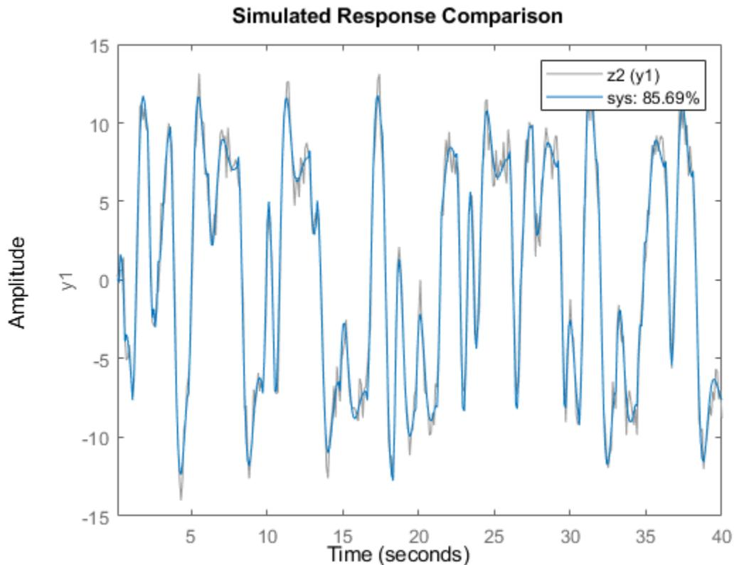
The fit of the simulated model to the measured data is nearly the same as the estimation fit.
