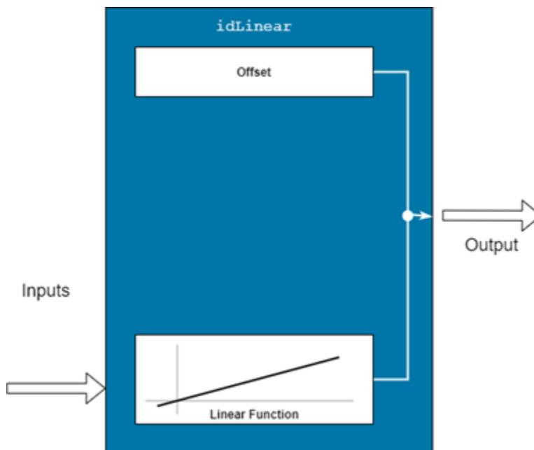
Mathematically, `idLinear` is a linear function  $y = F(x)$  that maps  $m$  inputs  $X(t) = [x(t_1), x_2(t), \dots, x_m(t)]^T$  to a scalar output  $y(t)$ .  $F$  is a (affine) function of  $x$ :
