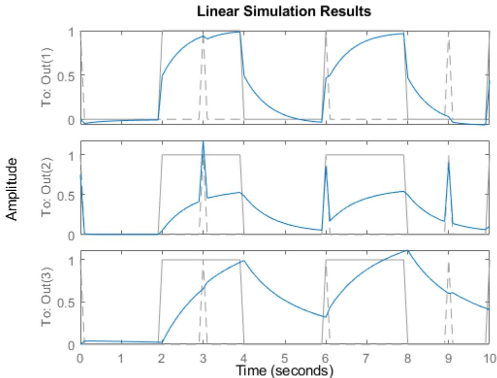
Each axis shows the response of one of the three system outputs to the signals  $u$  applied at all inputs. Each plot also shows all input signals in gray.
