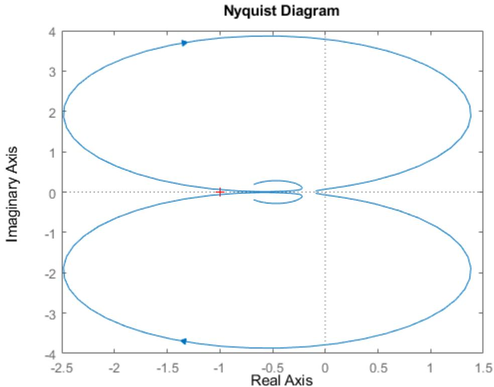
The cell array `{1, 100}` specifies a frequency range `[1,100]` for the positive frequency branch and `[-100,-1]` for the negative frequency branch in the Nyquist plot. The negative frequency branch is obtained by symmetry for models with real coefficients. When you provide frequency bounds in this way, the function selects intermediate points for frequency response data.
