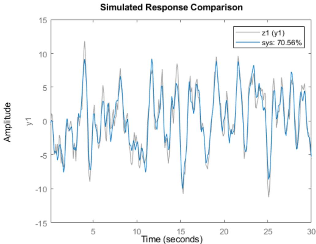
The plot illustrates the differences between the model response and the original data. The percentage shown in the legend is the NRMSE fitness value. It represents how close the predicted model output is to the data.
