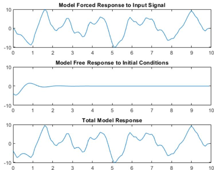
For continuous systems ( $T_s = 0$ ), the free response  $G(s)$  for the initial state vector  $x_0$  is
