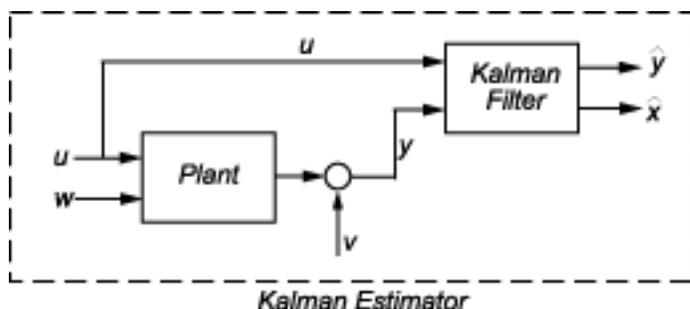
The block implements the steady-state Kalman filter when the system matrices ( $A(t)$ ,  $B(t)$ ,  $C(t)$ ,  $D(t)$ ,  $G(t)$ ,  $H(t)$ ) and noise covariance matrices ( $Q(t)$ ,  $R(t)$ ,  $N(t)$ ) are constant (specified in the Block Parameters dialog box). The steady-state Kalman filter uses a constant matrix  $P$  that minimizes the steady-state estimation error covariance and solves the associated continuous-time algebraic Riccati equation:
