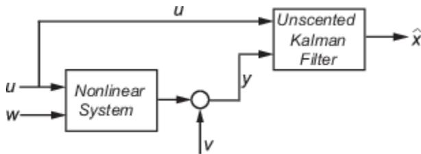
The algorithm computes the state estimates  $\hat{x}$  of the nonlinear system using state transition and measurement functions specified by you. The software lets you specify the noise in these functions as additive or nonadditive:
