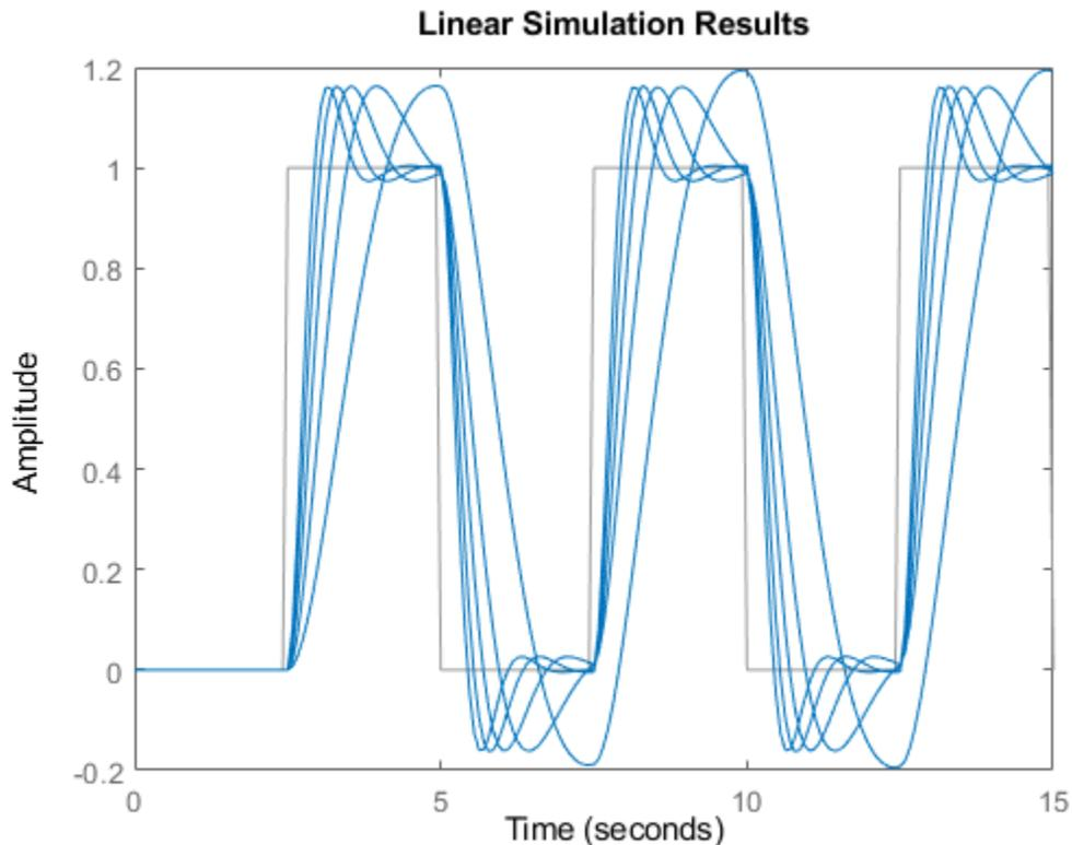
`lsim` uses the same line style for the responses of all entries in the array. One way to distinguish among entries is to use the `SamplingGrid` property of dynamic system models to associate each entry in the array with the corresponding  $w\theta$  value.
