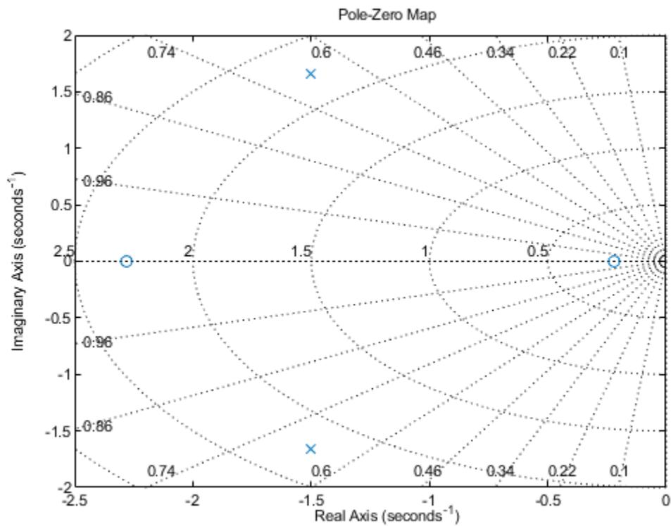
Turning on the grid displays lines of constant damping ratio (zeta) and lines of constant natural frequency ( $\omega_n$ ). This system has two real zeros, marked by o on the plot. The system also has a pair of complex poles, marked by x.
