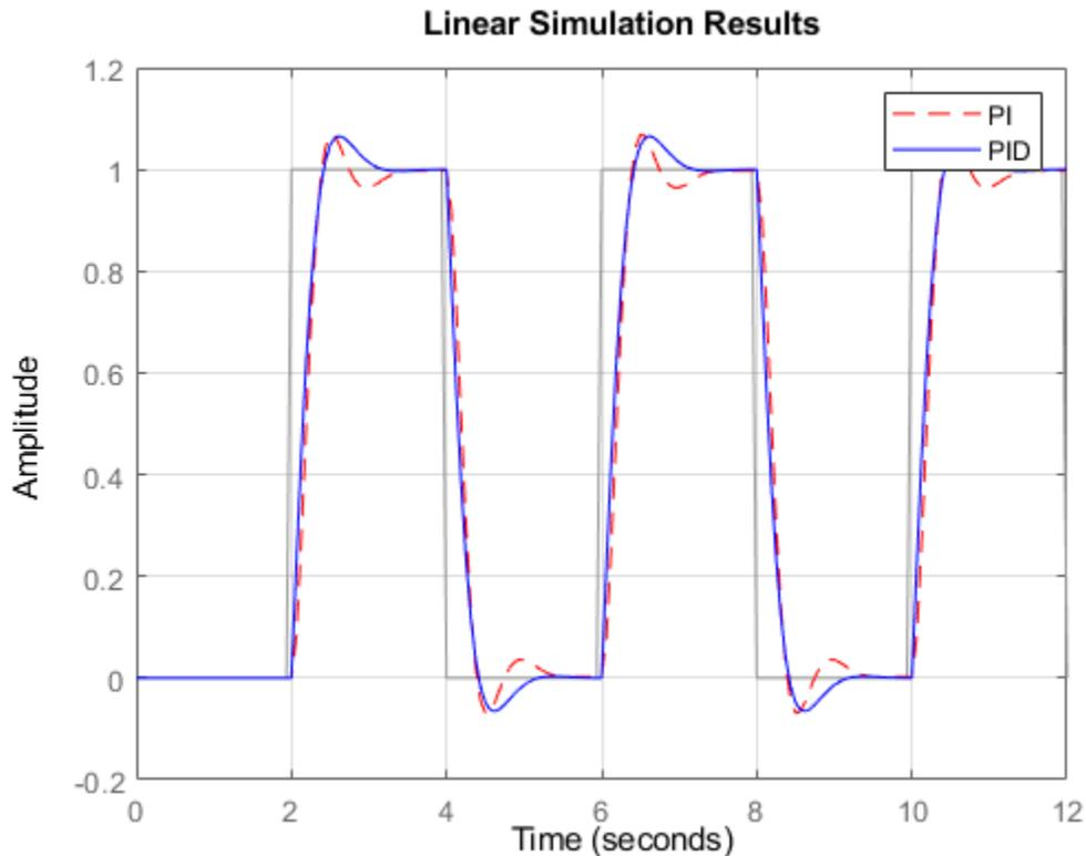
The first LineSpec "r - -" specifies a dashed red line for the response with the PI controller. The second LineSpec "b" specifies a solid blue line for the response with the PID controller. The legend reflects the specified colors and line styles. For more plot customization options, use `lsimplot`.
