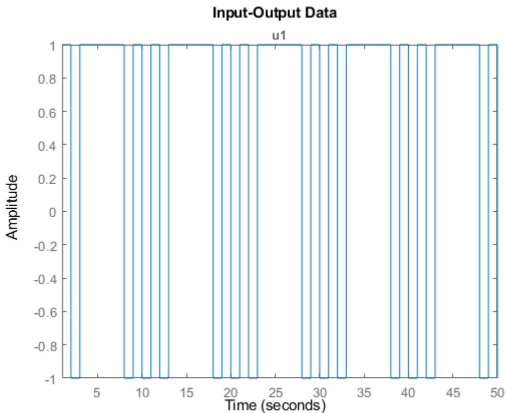
As specified, the generated single-channel periodic random binary input signal has a period of 10 seconds, and there are 5 whole periods in the signal.
