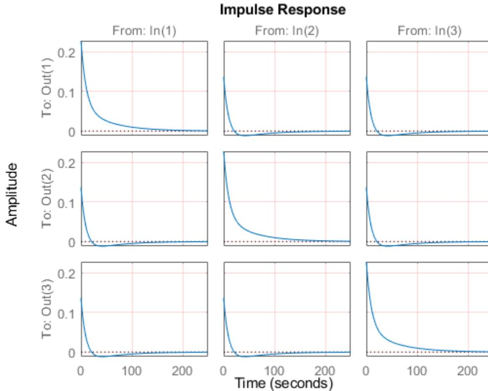
The impulse plot automatically updates when you call `setoptions`. For MIMO models, `impzplot` produces a grid of plots, each plot displaying the impulse response of one I/O pair.
