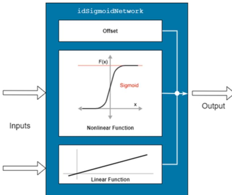
Mathematically, `idSigmoidNetwork` is a function that maps  $m$  inputs  $X(t) = [x_1(t), x_2(t), \dots, x_m(t)]^T$  to a scalar output  $y(t)$  using the following relationship:
