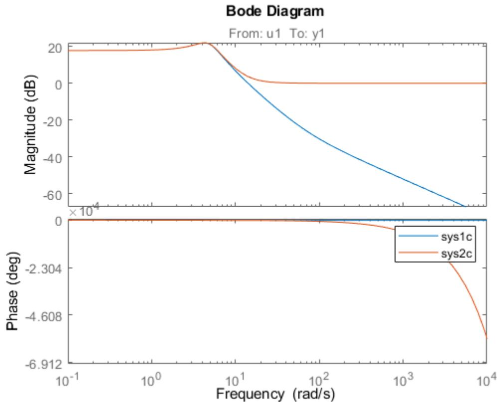
As the plot shows, the Bode responses of the two models do not match when you convert them to continuous time. When there is no feedthrough, as with `sys1c`, there must be some lag. When there is feedthrough, as with `sys2c`, there can be no lag. Continuous-time feedthrough maps to discrete-time feedthrough. Continuous-time lag maps to discrete-time delays.
