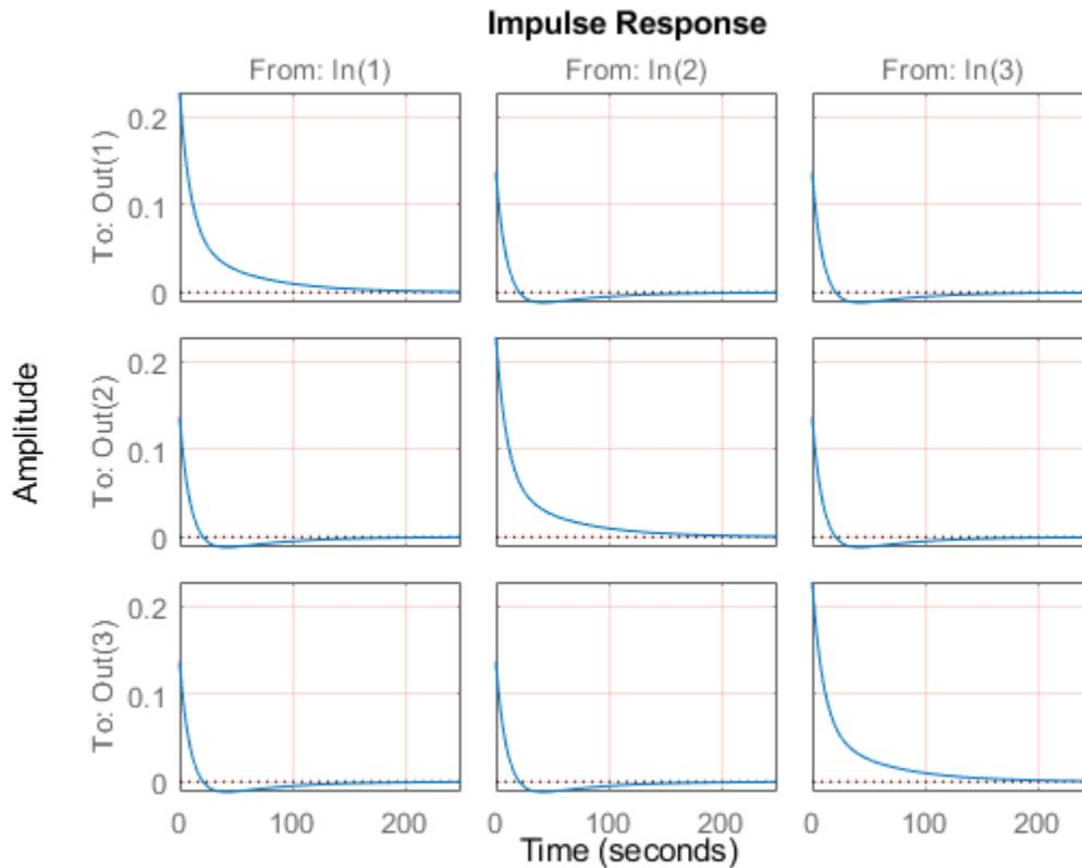
The impulse plot automatically updates when you call `setoptions`. For MIMO models, `impulseplot` produces a grid of plots, each plot displaying the impulse response of one I/O pair.
