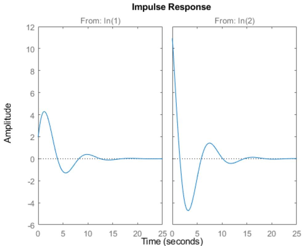
The left plot shows the impulse response of the first input channel, and the right plot shows the impulse response of the second input channel.
