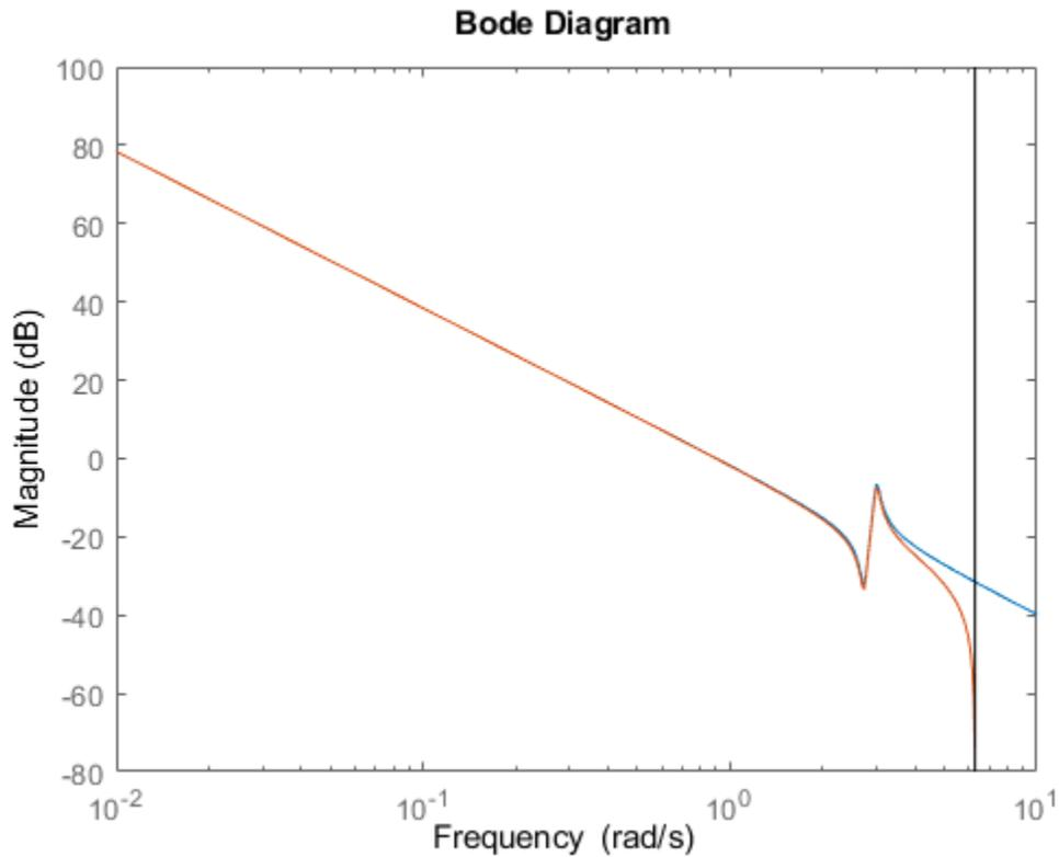
The Bode magnitude plot of a discrete-time system includes a vertical line marking the Nyquist frequency of the system.
