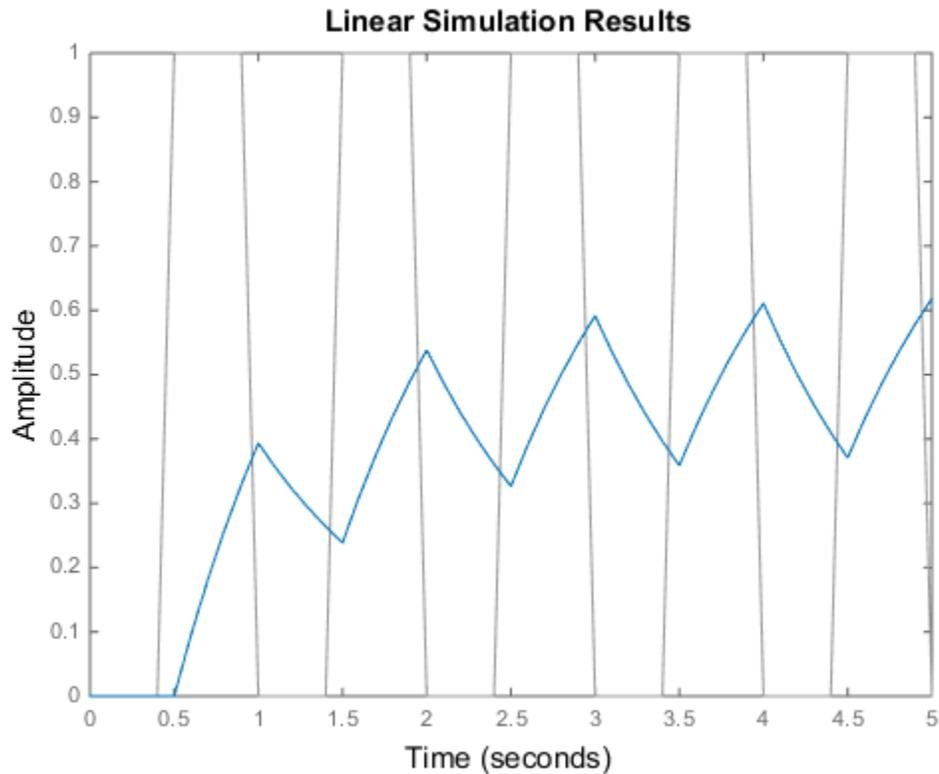
`lsim` simulates the model using the specified input signal, but it issues a warning that the input signal is undersampled. `lsim` recommends a sample time that generates at least 64 samples per period of the input `u`. To see why this recommendation matters, simulate `sys` again using a sample time smaller than the recommended maximum.
