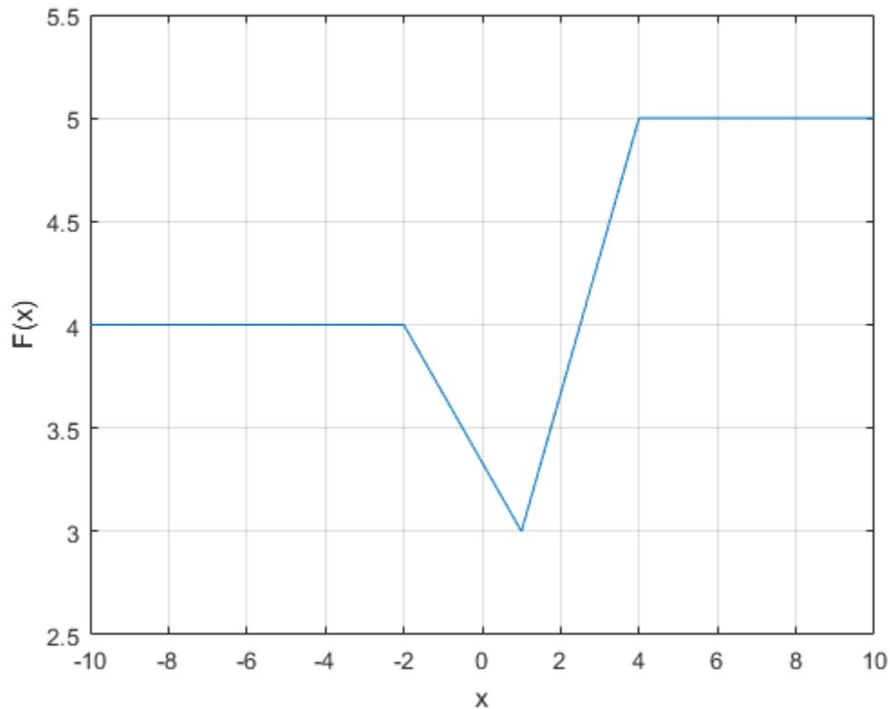
The value  $F(x)$  is computed by `evaluate(NL,x)`, where `NL` is the `idPiecewiseLinear` object. When using `evaluate`, the break points have to be initialized manually.
