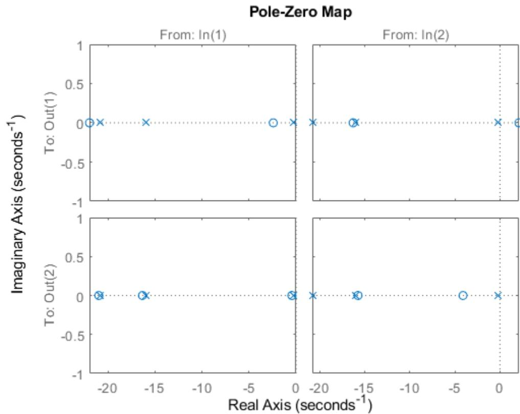
By default, the plot displays the poles and zeros of each I/O pair on its own axis. Use the plot handle to view all I/Os on a single axis.
