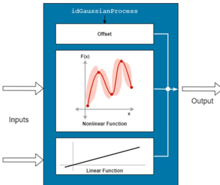
Mathematically, `idGaussianProcess` is a function that maps  $m$  inputs  $X(t) = [x(t_1), x_2(t), \dots, x_m(t)]^T$  to a scalar output  $y(t)$  using the following relationship:
