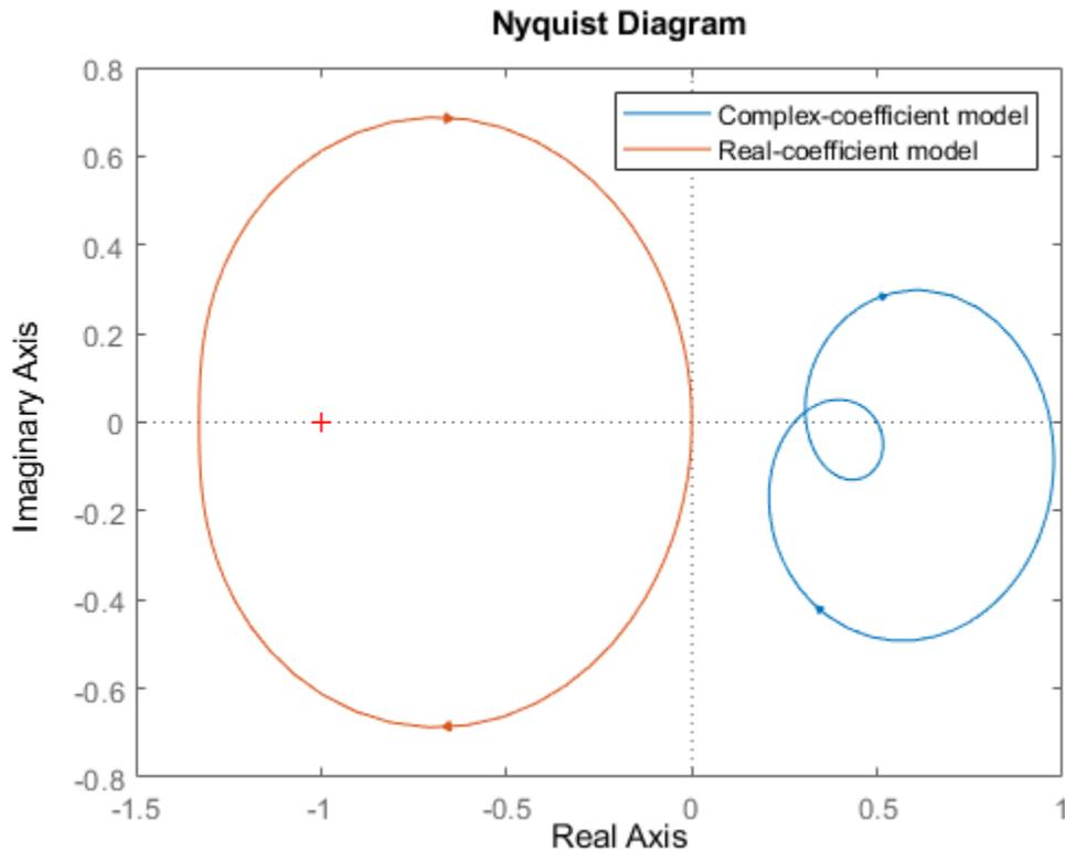
The Nyquist plot always shows two branches, one for positive frequencies and one for negative frequencies. The arrows indicate the direction of increasing frequency for each branch. For models with complex coefficients, the two branches are not symmetric. For models with real coefficients, the negative branch is obtained by symmetry.
