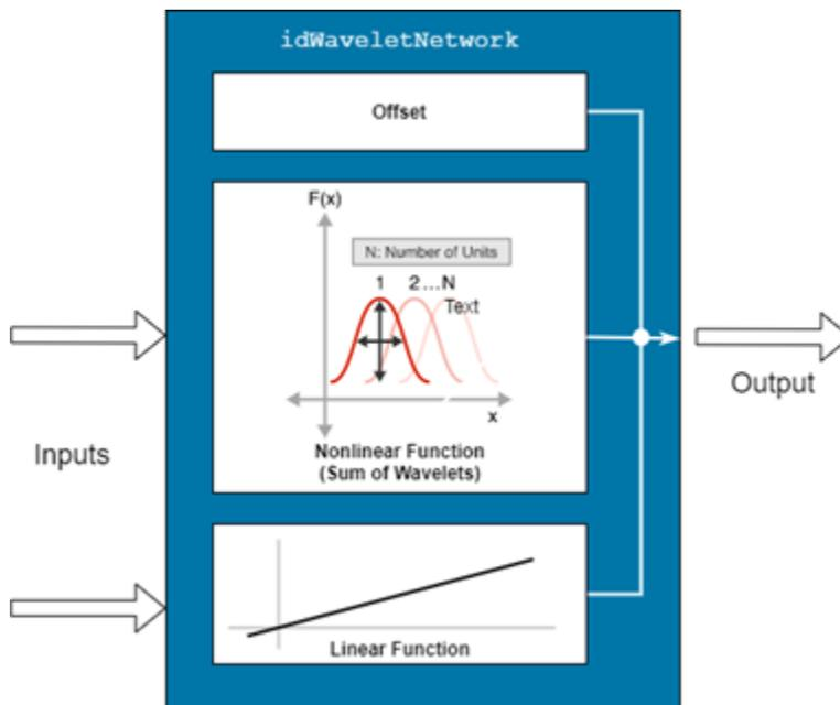
Mathematically, `idWaveletNetwork` is a function that maps  $m$  inputs  $X(t) = [x_1(t), x_2(t), \dots, x_m(t)]^T$  to a scalar output  $y(t)$  using the following relationship:
