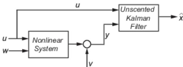
Using the state transition and measurement functions of the system and the unscented Kalman filter algorithm, the block produces state estimates  $\hat{x}$  for the current time step. For information about the algorithm, see “Extended and Unscented Kalman Filter Algorithms for Online State Estimation”.
