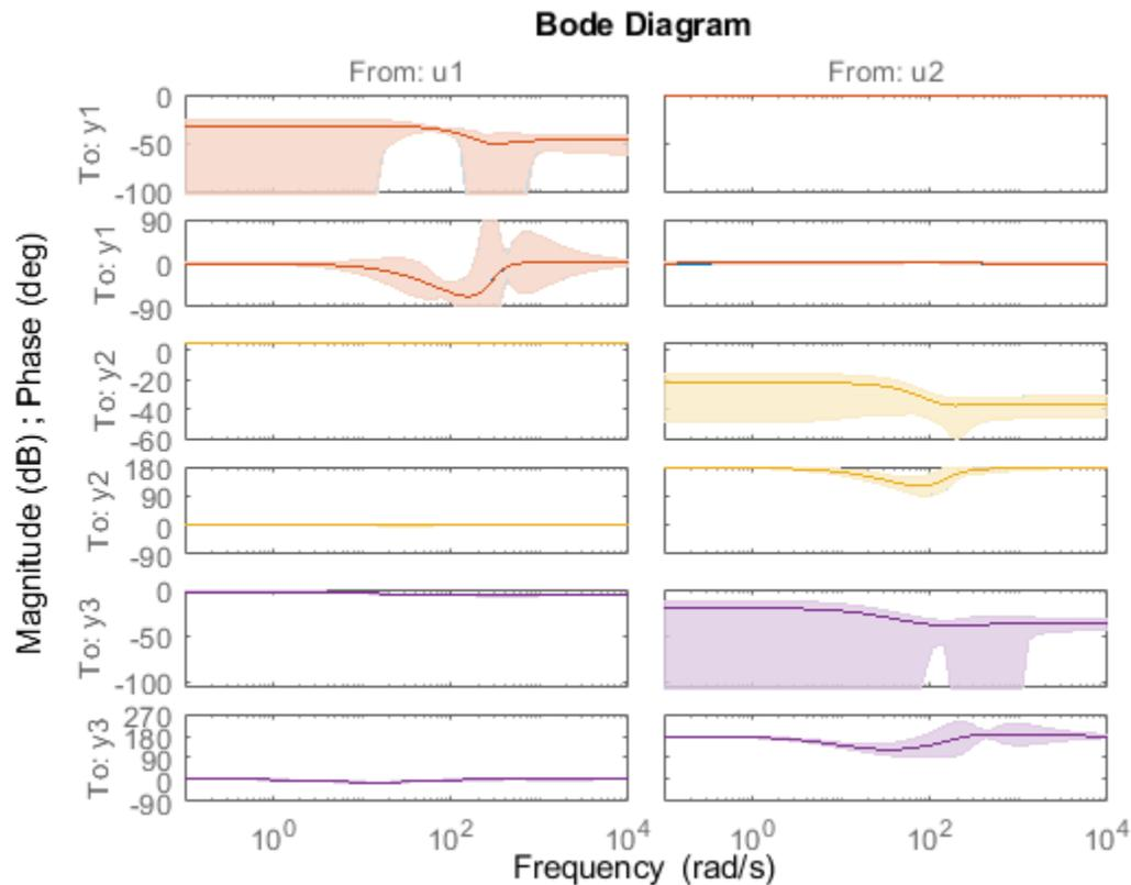
The confidence bounds for M2 overlap with those of m1, m2 and m3 models on their respective plot axes.
