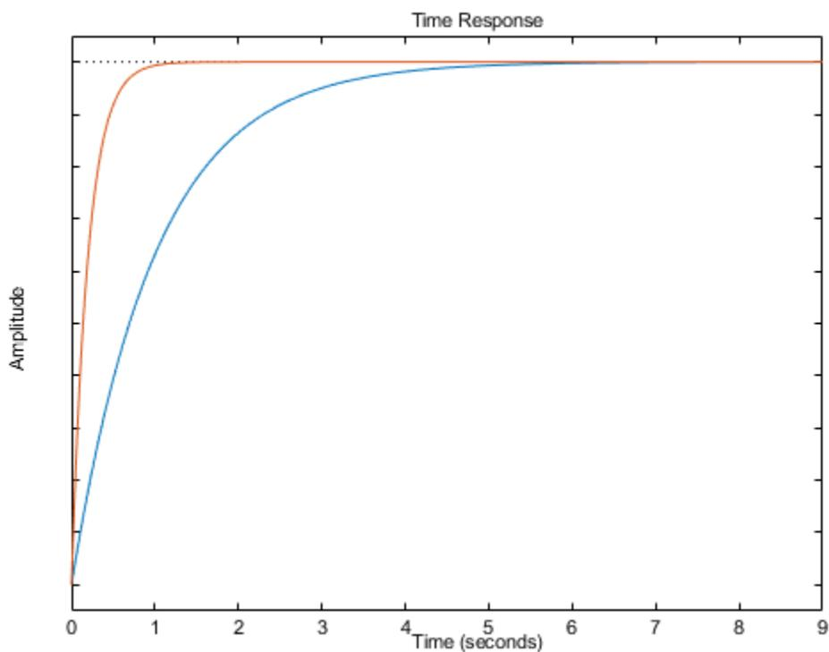
The plot shows the normalized step response for the two transfer function models.
