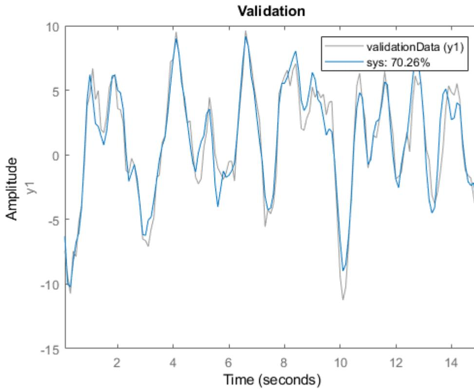
The fit to the estimation data is somewhat worse than in “Estimate Process Model with Live Editor Task” on page 1-288. Estimation in the current example has only half the data with which to estimate the model. The fit to the validation data, which represents the goodness of the model more generally, is better than the fit to the estimation data.
