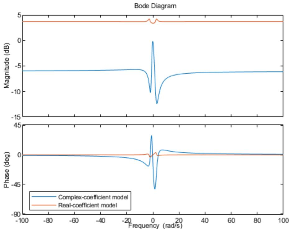
In linear frequency scale, the plot shows a single branch with a symmetric frequency range centered at a frequency value of zero. The plot also shows the negative-frequency response of a real-coefficient model when you plot the response along with a complex-coefficient model.
