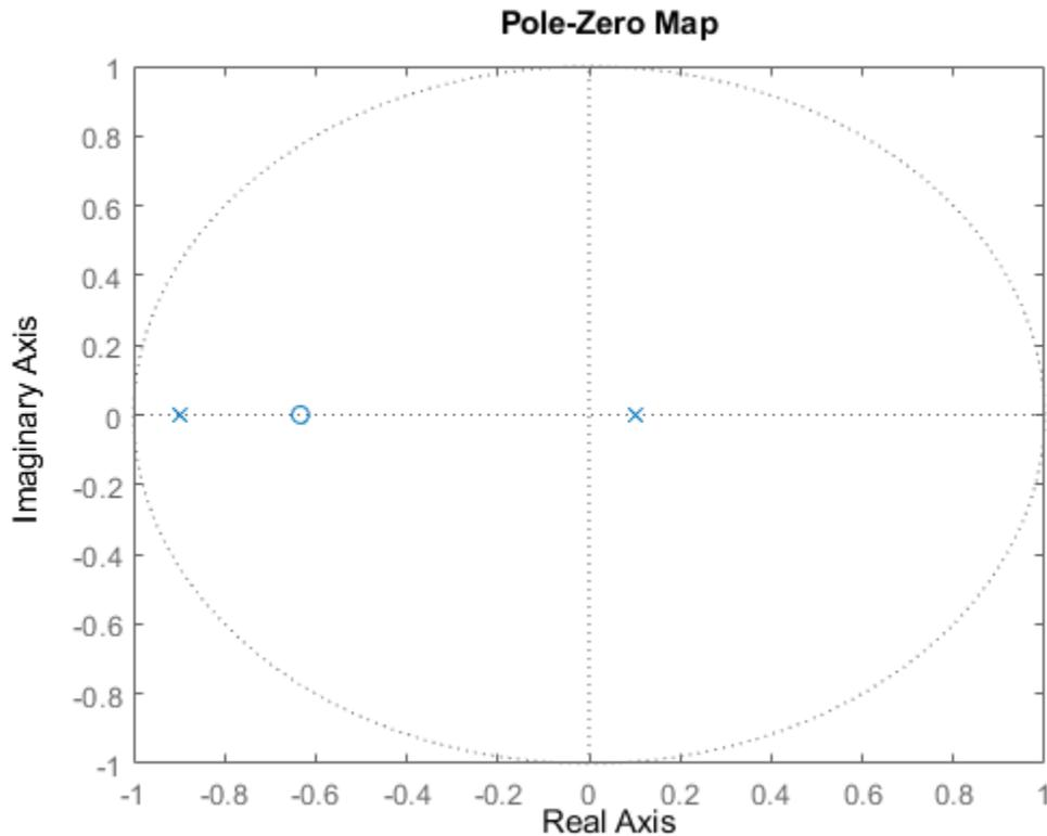
System poles are marked by x, and zeros are marked by o.
