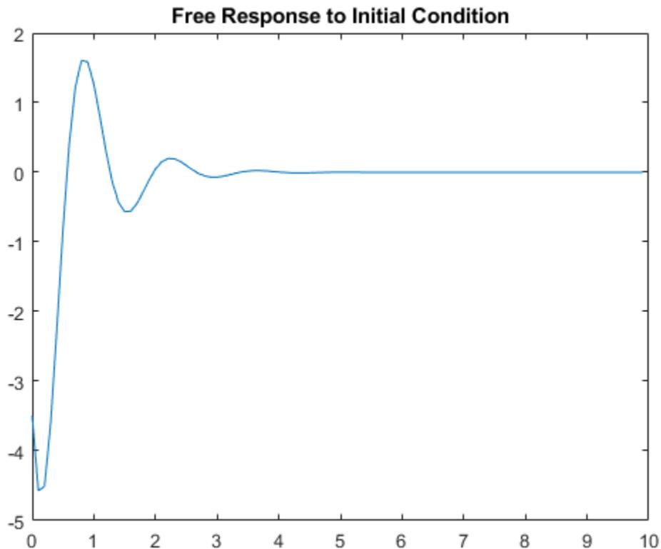
The free response is a transient that lasts for about four seconds.
