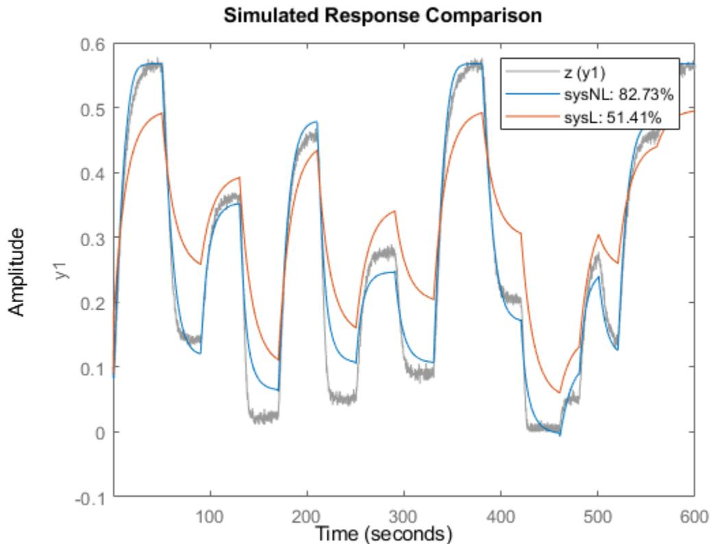
The nonlinear model has a much better fit to the data than the linear model.
