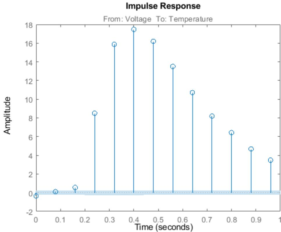
The first response value that is significantly different than zero occurs at 0.24 seconds, or the third sample. This implies that the transport delay is three samples. To generate a model that imposes the three-sample delay, set the transport delay, which is the third argument, to 3. You must also set the second argument, the order  $n$ , to its default value of `[]` as a placeholder.
