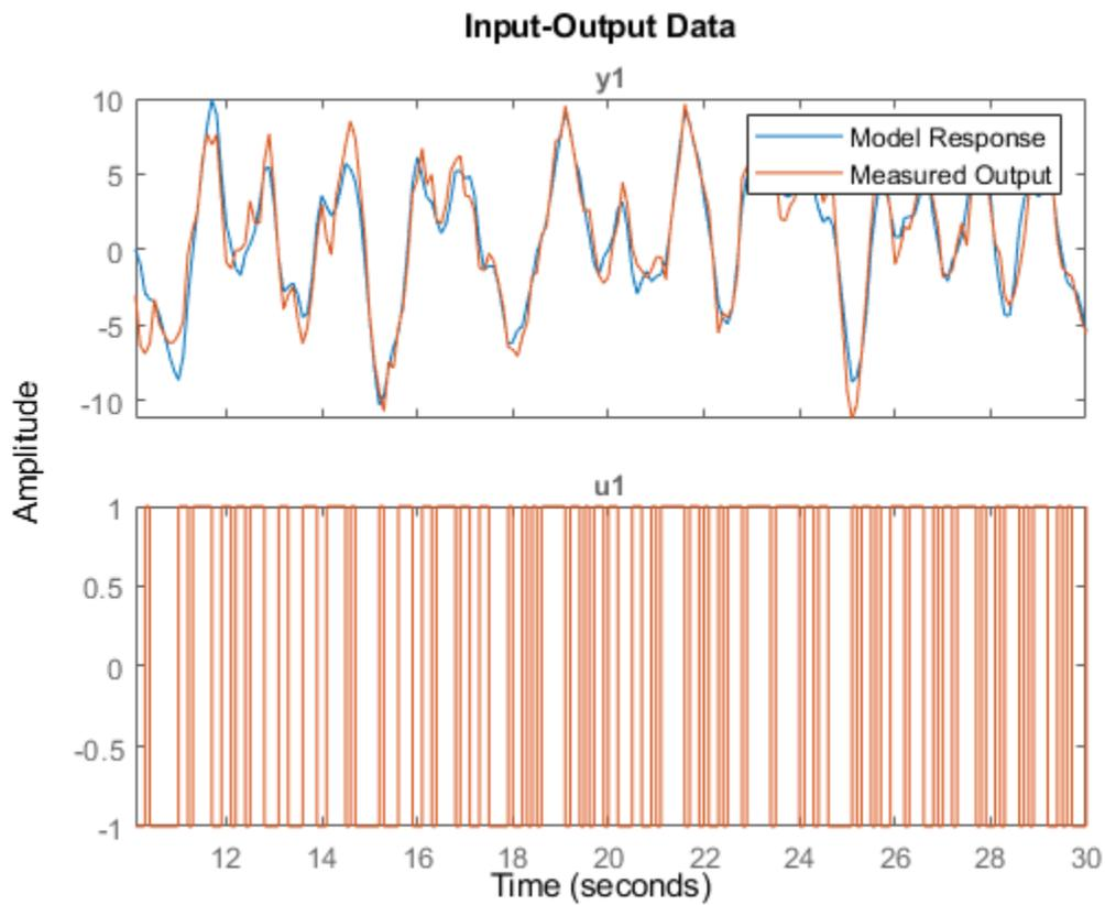
The measured and simulated outputs do not agree at the beginning of the simulation.
