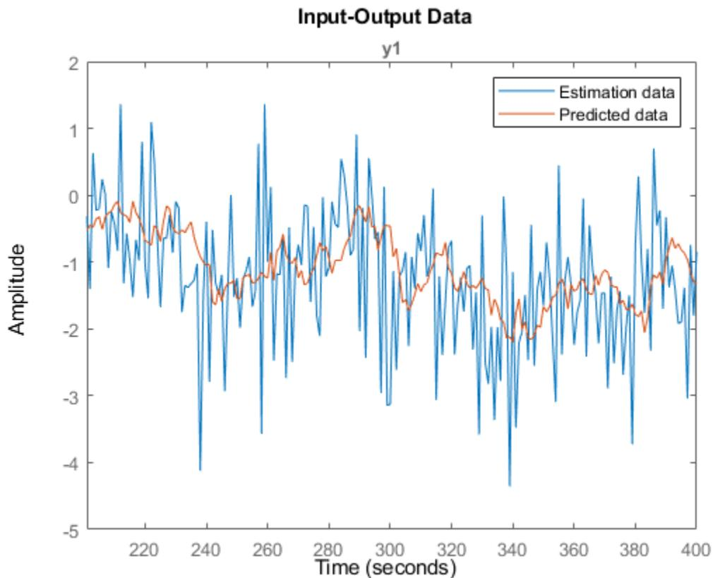
Alternatively, to plot the predicted response and estimation data, use `compare(sys, data, K)`.
