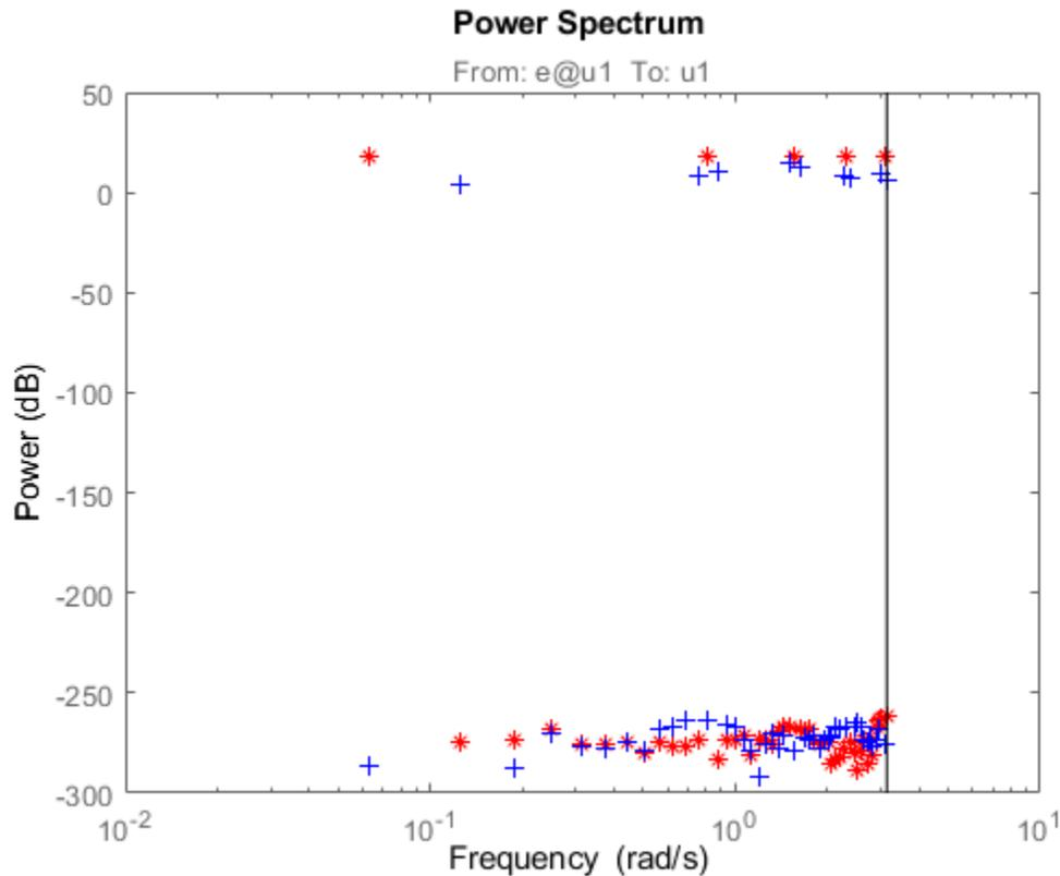
The plot shows some frequency splitting where the u2-based spectrum does not line up with the u1-based spectrum, but instead, contains two spectral points that flank certain u1-based points. This indicates the nonlinearity of the squared system.
