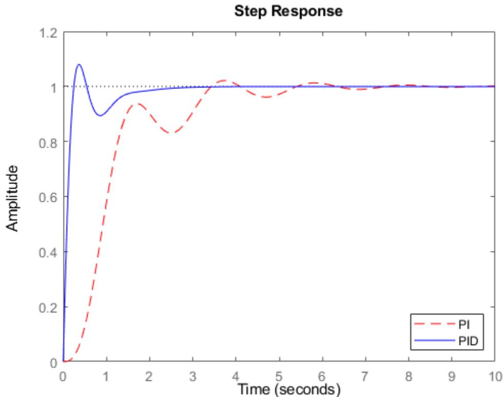
The first LineSpec 'r--' specifies a dashed red line for the response with the PI controller. The second LineSpec 'b' specifies a solid blue line for the response with the PID controller. The legend reflects the specified colors and linestyles. For more plot customization options, use `stepplot`.
