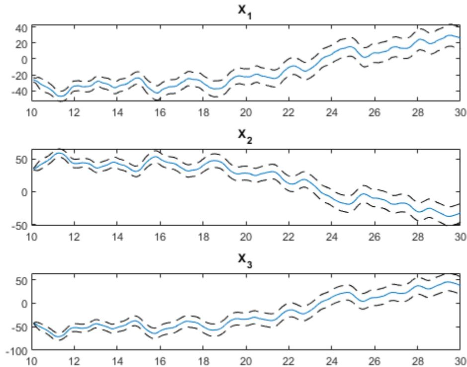
The response uncertainty does not grow over the forecasting time span because of the specification of future inputs.
