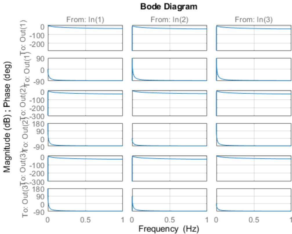
The Bode plot automatically updates when you call `setoptions`. For MIMO models, `bodeplot` produces an array of Bode plots, each plot displaying the frequency response of one I/O pair.
