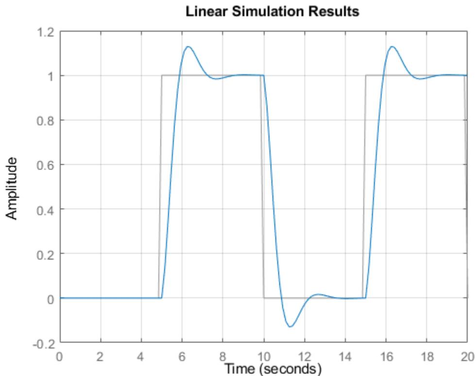
The plot shows the applied square wave in gray and the system response in blue. Call `lsim` with an output argument to obtain the response values at each point in `t`.
