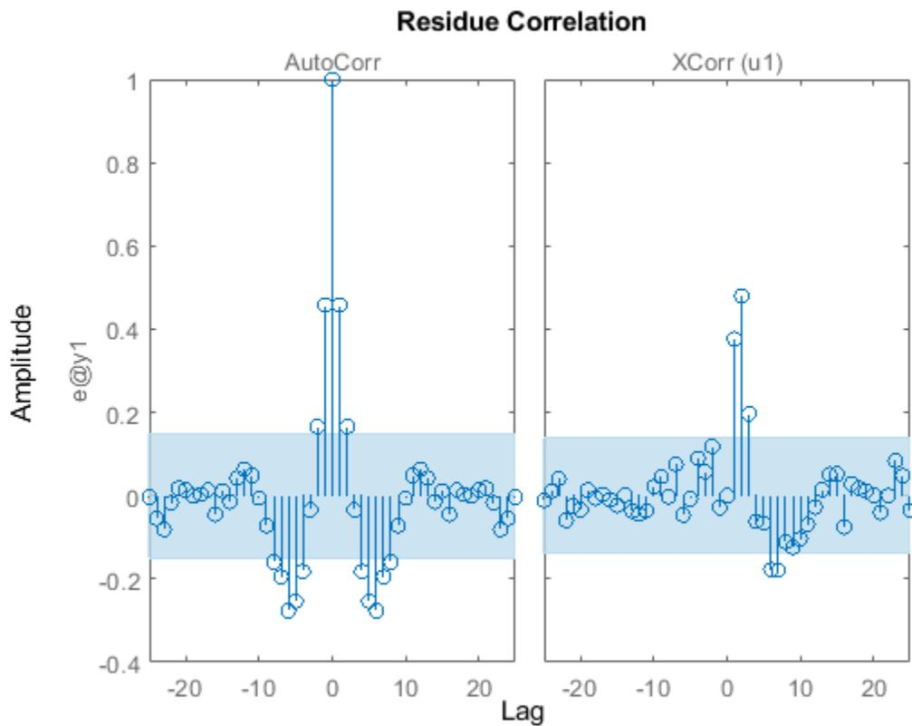
The correlations are calculated until the default maximum lag, 25. The 99% confidence region marking statistically insignificant correlations displays as a shaded region around the X-axis.
