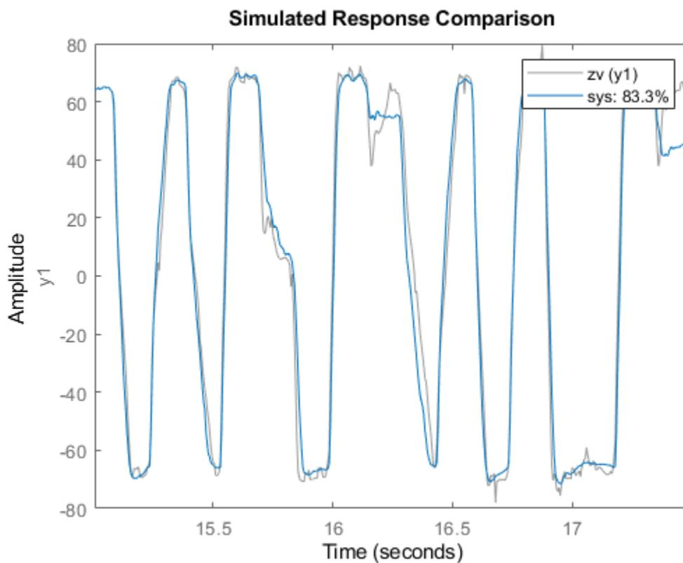
sys shows a good fit to both the estimation data and the validation data.
