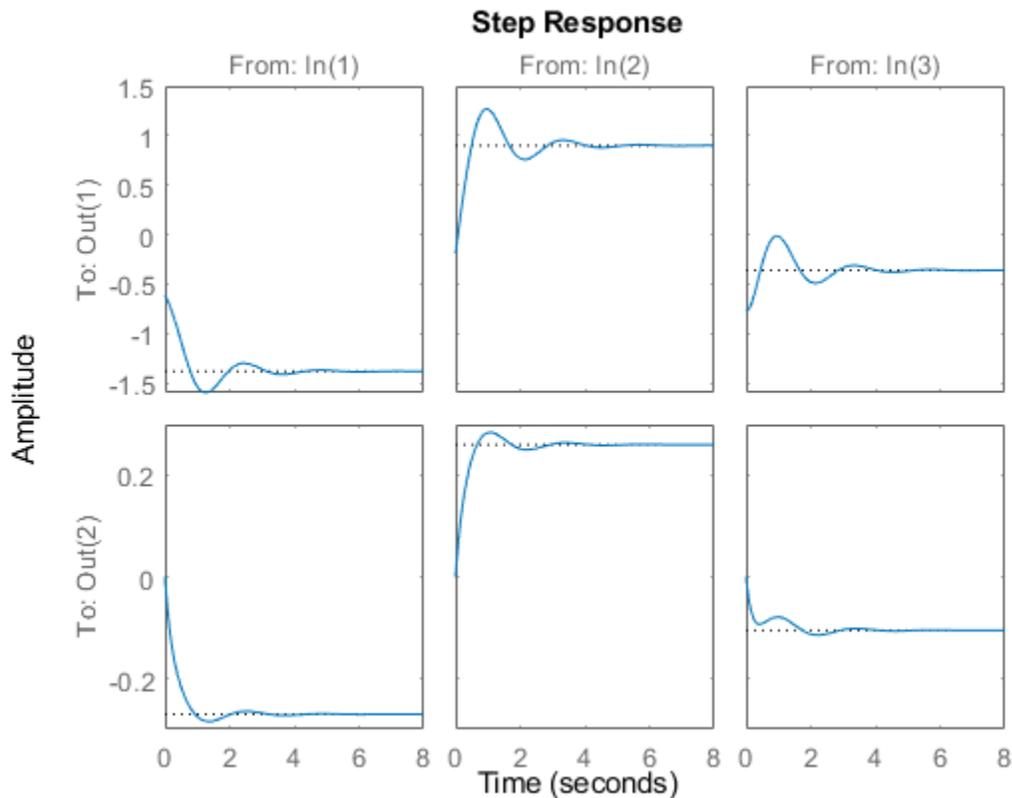
In a MATLAB figure window, you can restrict the plot to a subset of channels by right-clicking on the plot and selecting **I/O Selector**.
