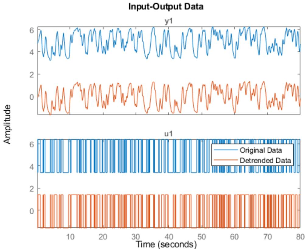
The detrended data has shifted by about 5 units. Inspect `Tr` to obtain the precise mean values that `detrend` computed and subtracted. These values are returned in the `InputOffset` and `OutputOffset` properties.
